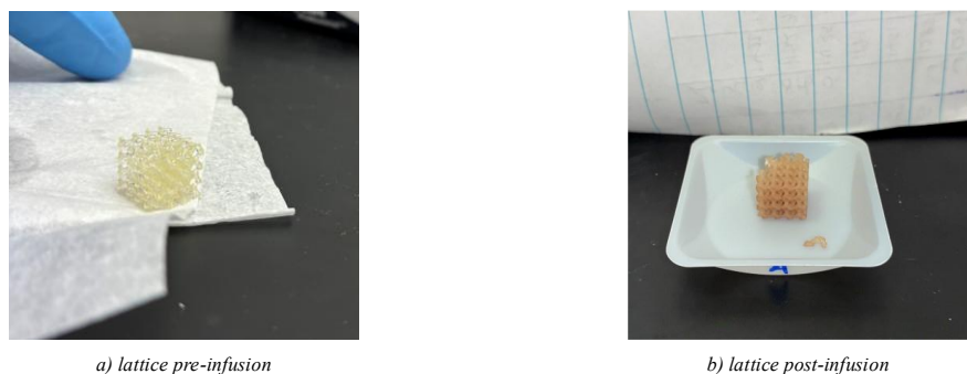
Figure 6-3: Photograph of gyroid lattice before infusion (clear/white) and after infusion (yellow-orange coloration from \text{Ce}^{3+} ions)
