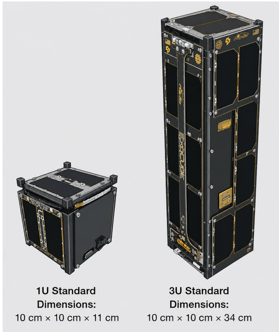
Figure 17. A 1U CubeSat was the first satellite developed at Cal Poly to qualify a reliable bus system, sensors and attitude control devices (left), a 3U CubeSat, was also designed at Cal Poly with space weather sensors from NASA's Goddard Space Flight Center (right). Source: [(NASA CubeSat Launch Initiative, 2017)]
