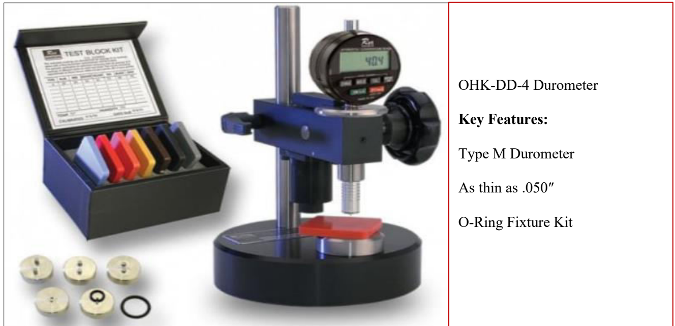
Figure 5. 8: Hardness analysis of aged sealing samples
