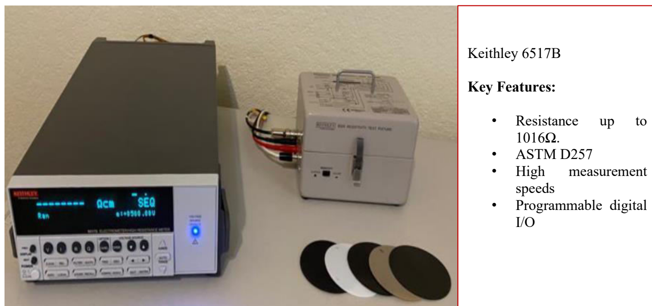
Figure 5. 9: Resistivity analysis of aged sealing samples
