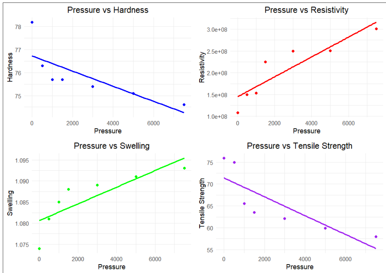
Figure 6. 27: Interaction of pressure on material properties of NBR
