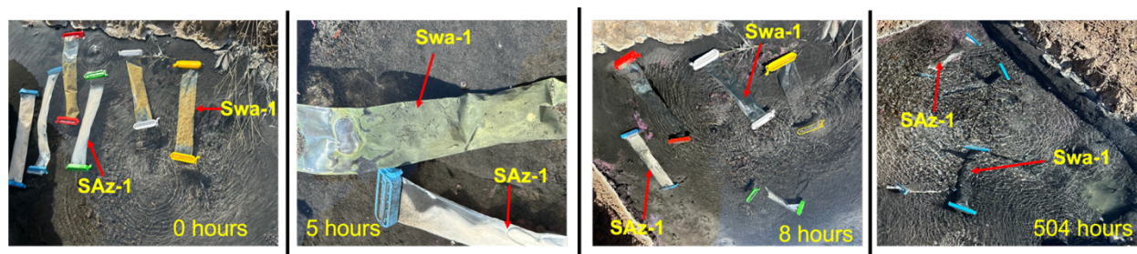
Figure 1: Smectite color change with respect to reaction time in the spring. Only Fe-rich SWa-1 shows intense color change with increasing reaction time.
