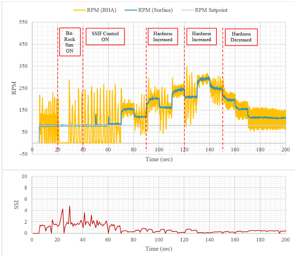
Figure 65. SSIF controller response in vertical well configuration (0.3-0.5 SSI thresholds, 1000g hook load)
