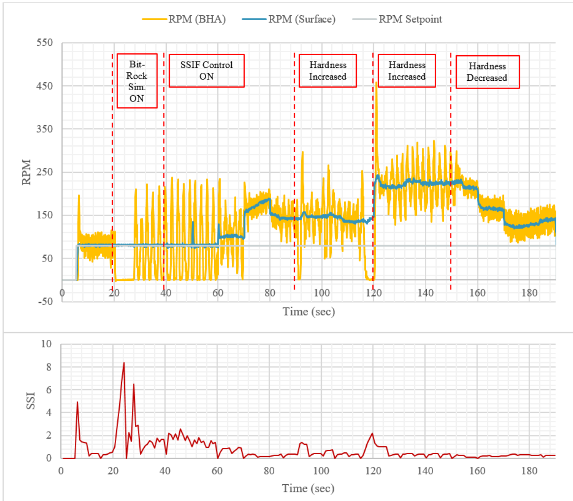
Figure 66. SSIF controller response in vertical well configuration (0.3-0.5 SSI thresholds, 1500g hook load)
