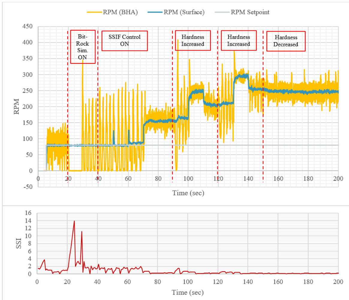
Figure 63. SSIF controller response in vertical well configuration (0.2-0.4 SSI thresholds, 1000g hook load)
