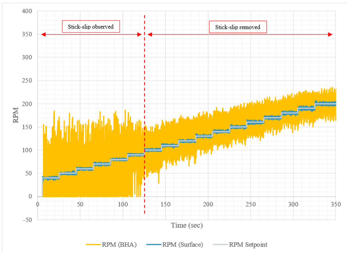
Figure 57. Feedback RPM control in vertical well configuration
