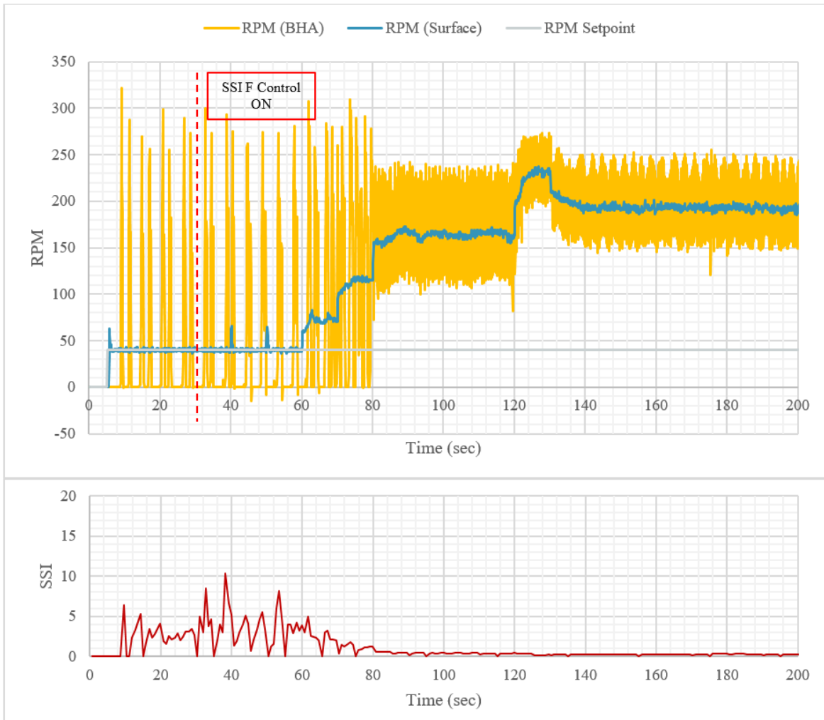
Figure 69. SSIF controller response in directional well configuration (0.2-0.4 SSI thresholds, 1000g hook load)
