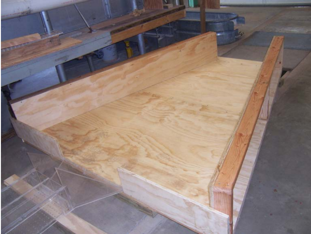
Figure 14. Downstream plywood channel after wingwall.
