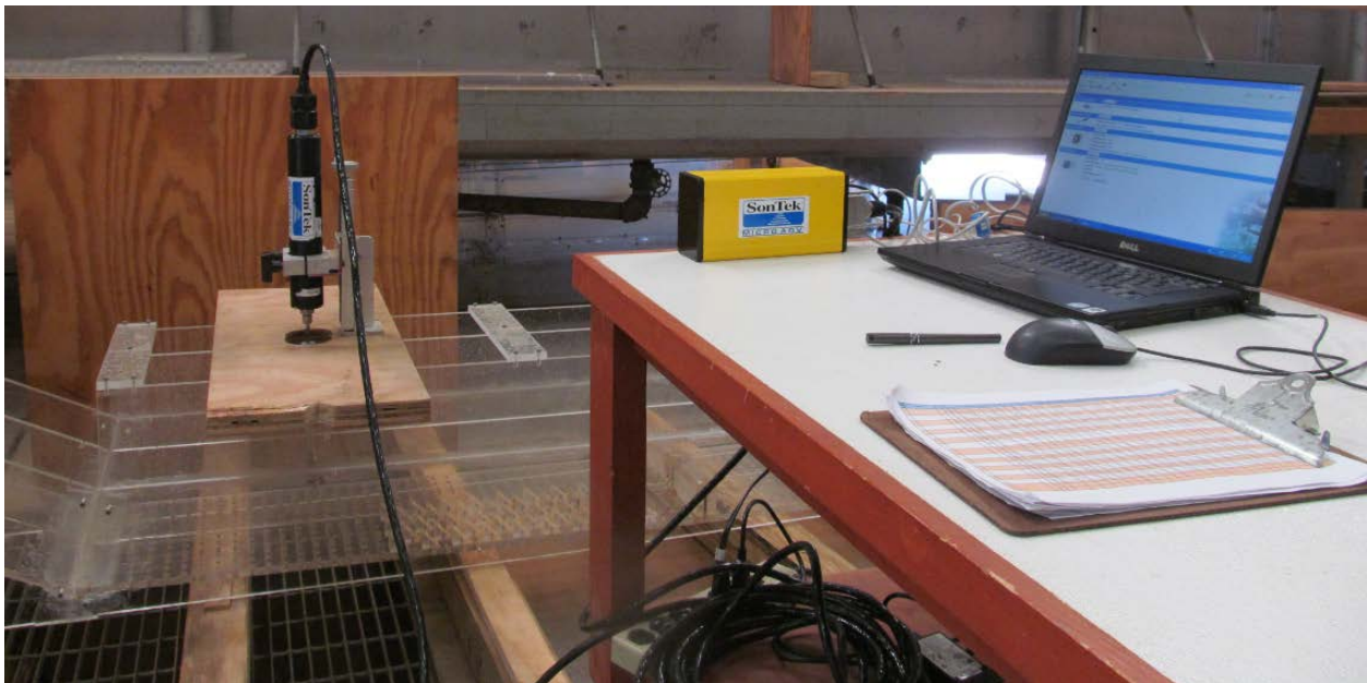
Figure 17. ADV plugged in the culvert model connected with the computer
