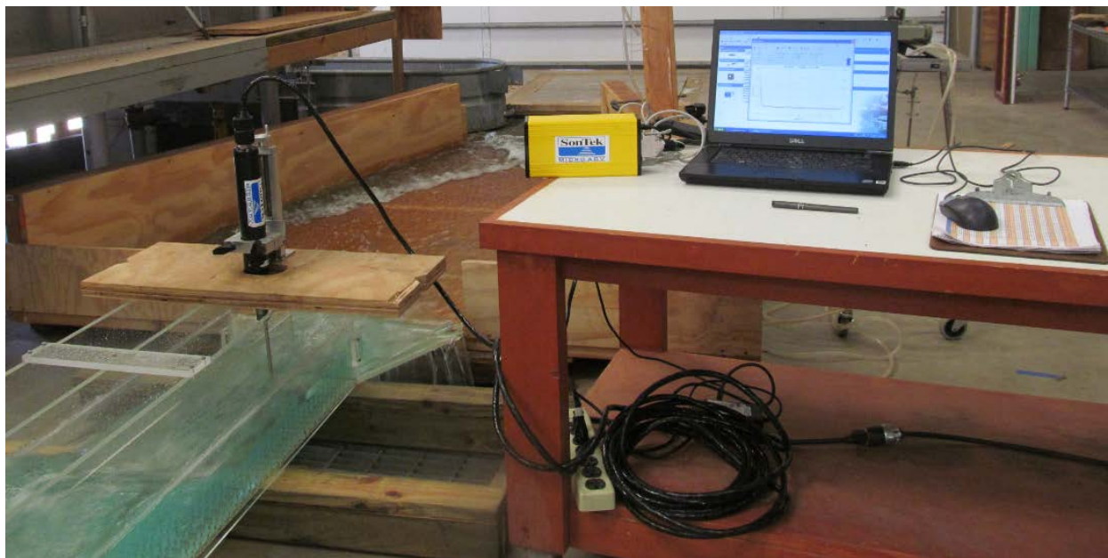
Figure A113. ADV plugged to measure the downstream velocity V_{d/s}
