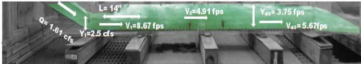
Figure 24. Hydraulic jump characteristics for Experiment 29C for 0.6% slope, 1.2d.
