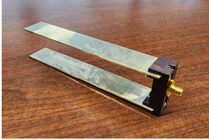
Figure 3.25: Fabricated plate assembly with 3D-printed spacer used to support structure and SMA connector used to feed a signal to the plates.
