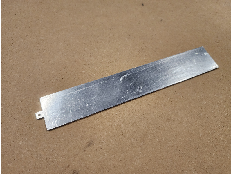
Figure 3.18: Fabricated aluminum plate based on the revised design dimensions from Table 3.3, incorporating changes such as a reduced feed size to improve field confinement and response.
