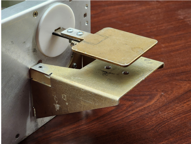
Figure 3.8: Original parallel plate structure connected to the Comdel MatchPro CPMX-6000. The RF signal is fed through the housing to the top plate, while the bottom plate is grounded to the chassis, creating an electric field between plates.
