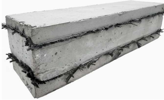
Figure 17: CFRP reinforced manual fabrication
