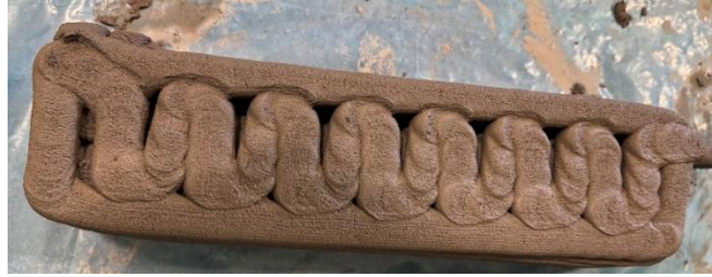
Figure 53: 3D printed non-reinforced specimens
