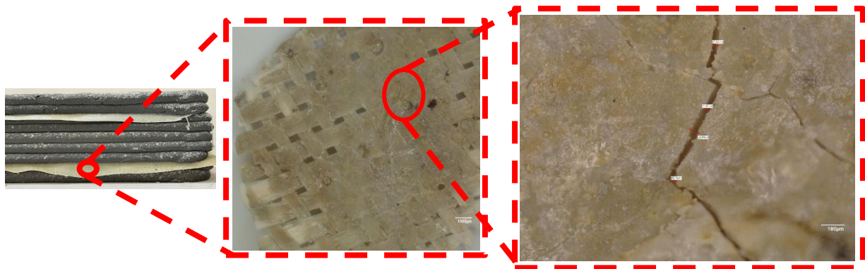
Figure 85: Microscopic investigation of 60 days exposed GFRP+Resin specimen focusing on reinforcement deterioration
