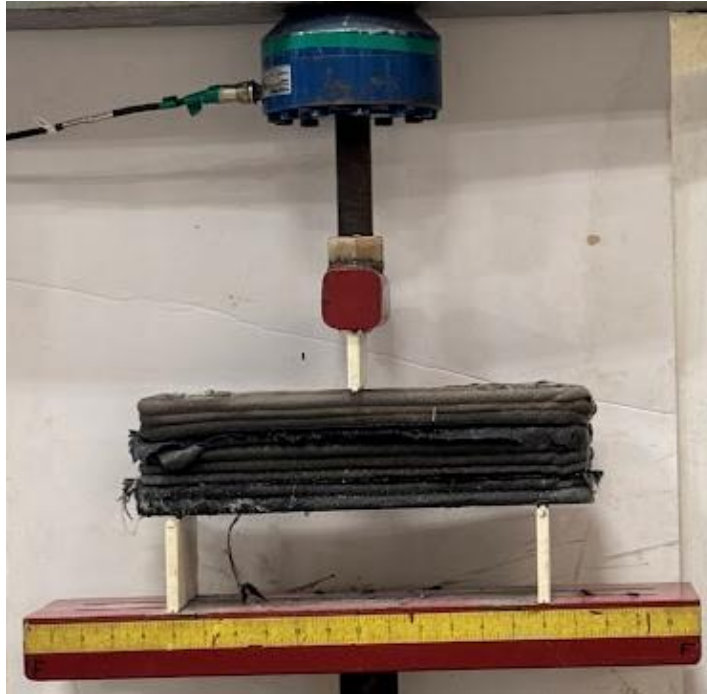
Figure 71: Experimental setup for 3D Printed CFRP specimen under MTS frame
