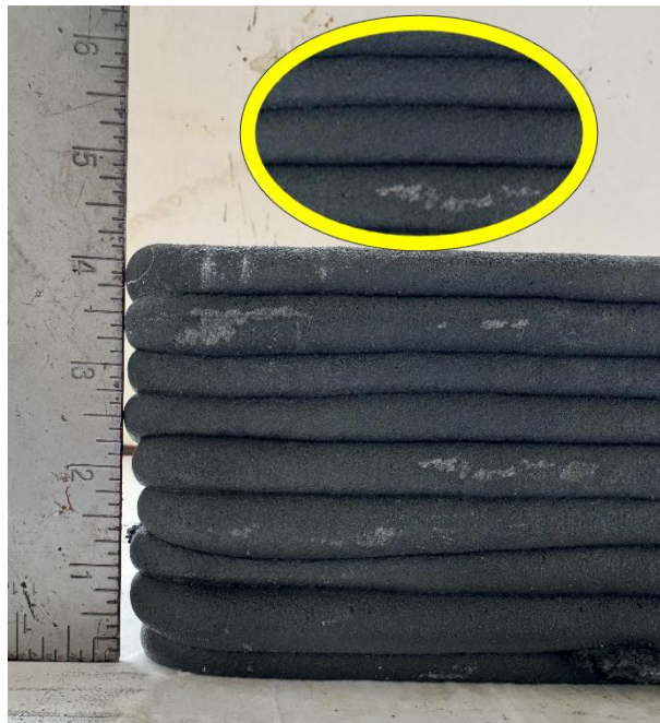
Figure 54: 3D Printed non-reinforced layer thickness and height
