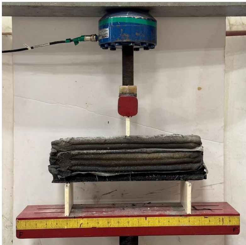
Figure 74: Experimental setup for 3D Printed Steel specimen under MTS frame
