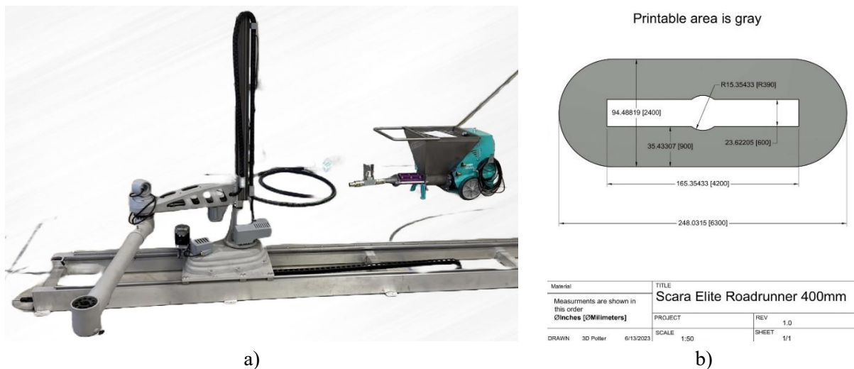
Figure 42: (a) Scara Elite Roadrunner 4M with extruder pump, (b) Plan view of printer with dimensions
