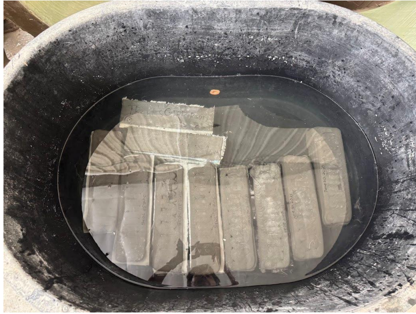
Figure 64: Chemical ingress chamber with 6% NaCl and \text{pH} < 2
