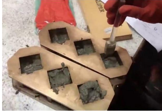
Figure 13: 50mm x 50mm cementitious cube preparation
