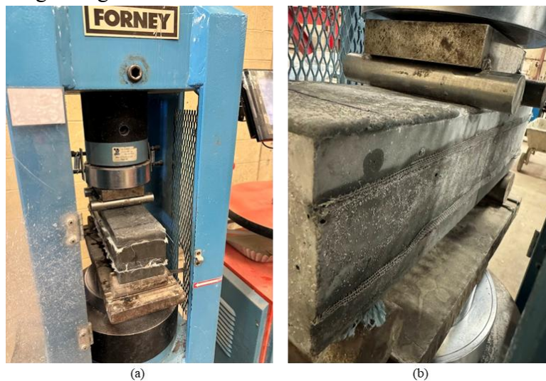
Figure 22: (a) Forney flexural testing setup, (b) 4-point bending test setup
