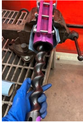
Figure 61: Rotor (pink) and Stator (black spiral rod)
