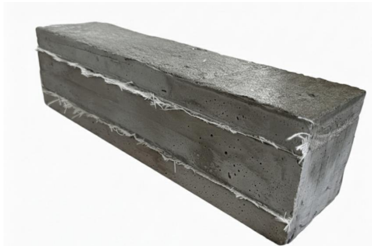
Figure 18: GFRP reinforced manual fabrication
