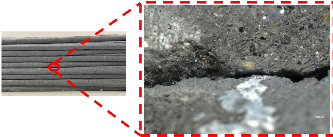
Figure 86: Microscopic investigation of 60 days unexposed non-reinforced specimen focusing on the layer
