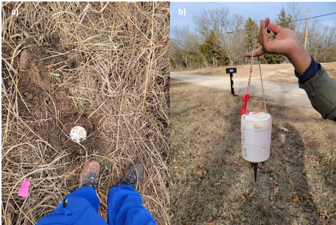
Figure 21: Deploying nodes to collect aftershocks of the 2024 M_w 5.1 earthquake in Prague, OK with OGS. a) Buried node b) Node used to collect aftershock data.
