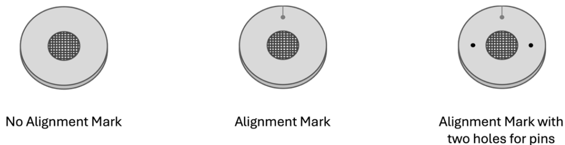
Figure 2.15: Button orientation marker evolution: The first button prototype started out with no alignment markers. Once spectral changes due to button orientation were noted, an alignment mark was added as in the middle button. This alignment
