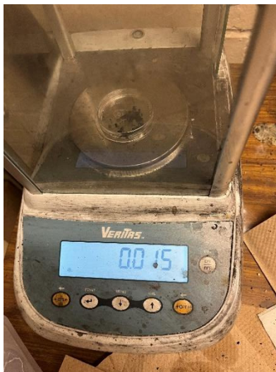
Figure 29: Picture Showing Measurement Of 15mg of CNT
