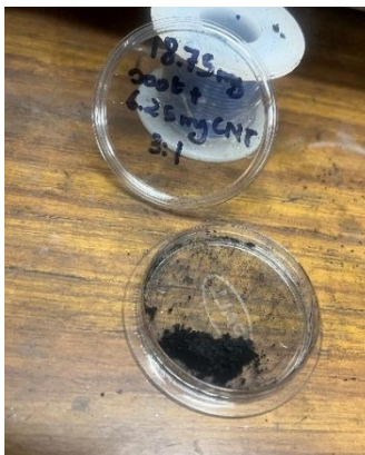
Figure 30: Picture Displaying A 3:1 Ratio of Soot to CNT
