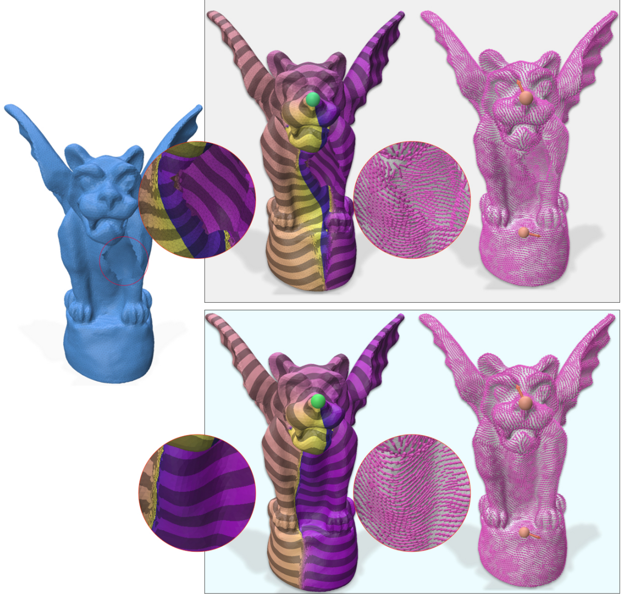
Figure 5.9: Surface PDE continuation on repaired meshes. Top: the input mesh with holes. Bottom: the repaired mesh. Logarithmic map and parallel transport are computed directly on the repaired surface by reusing boundary conditions along the hole edges.
