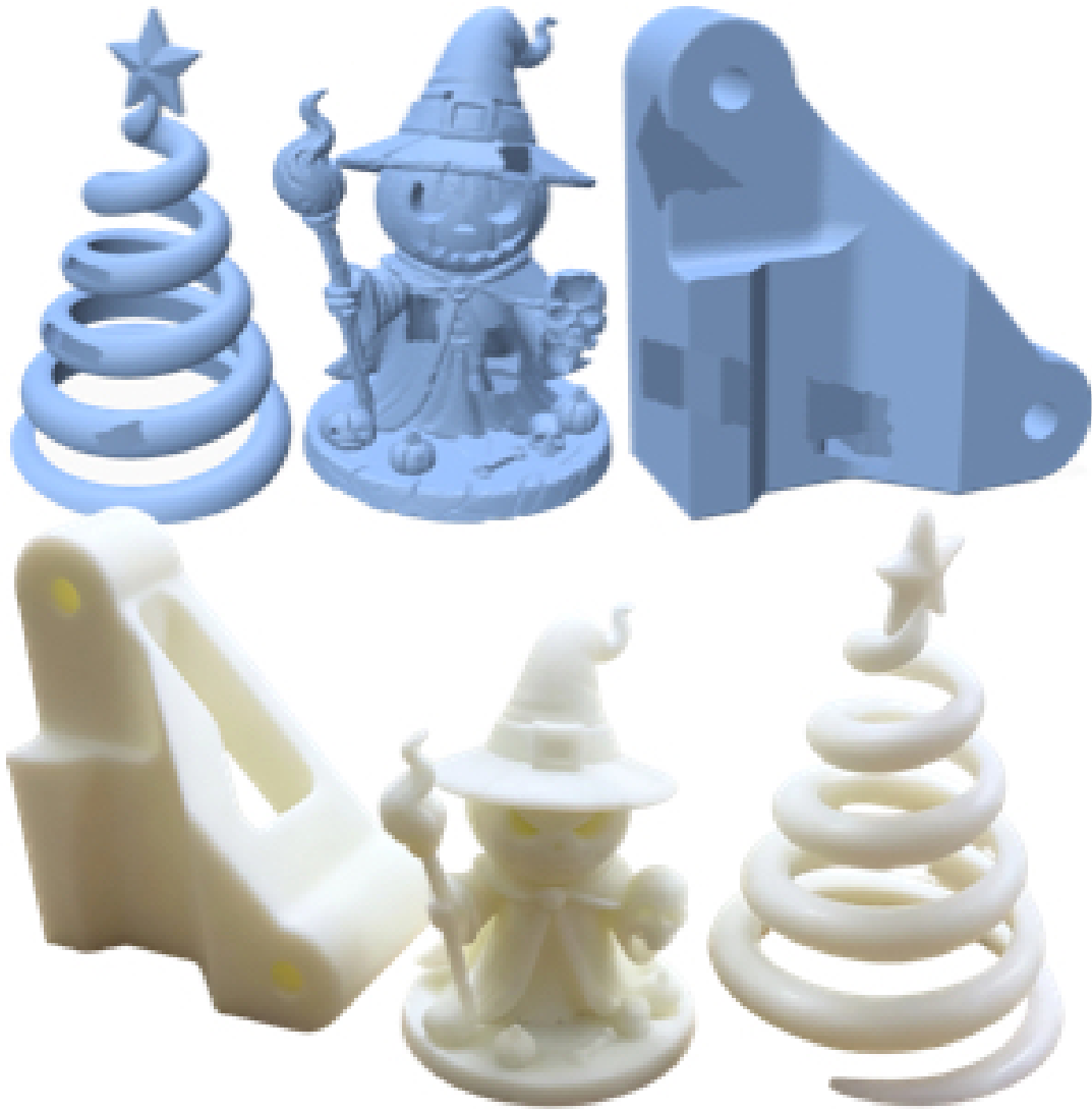
Figure 5.10: Repaired meshes from our method are watertight and structurally sound, allowing direct 3D printing without additional post-processing or remeshing.
