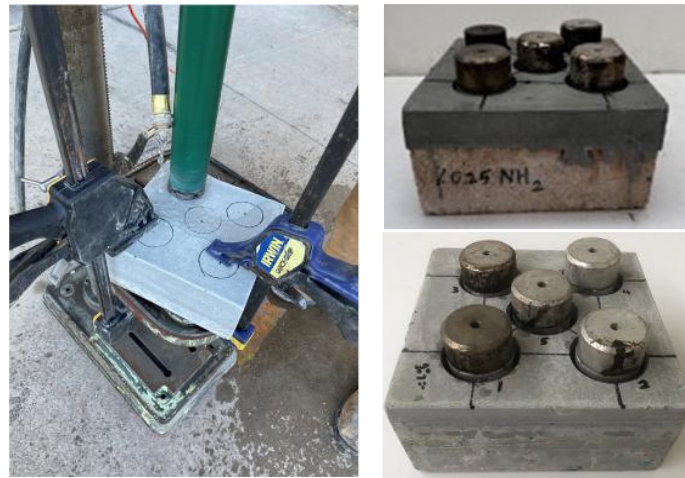
Figure 27: Preparation of the test specimens for the pull-off method (left–right), drilling cores, and the attachment of tensile loading devices.
