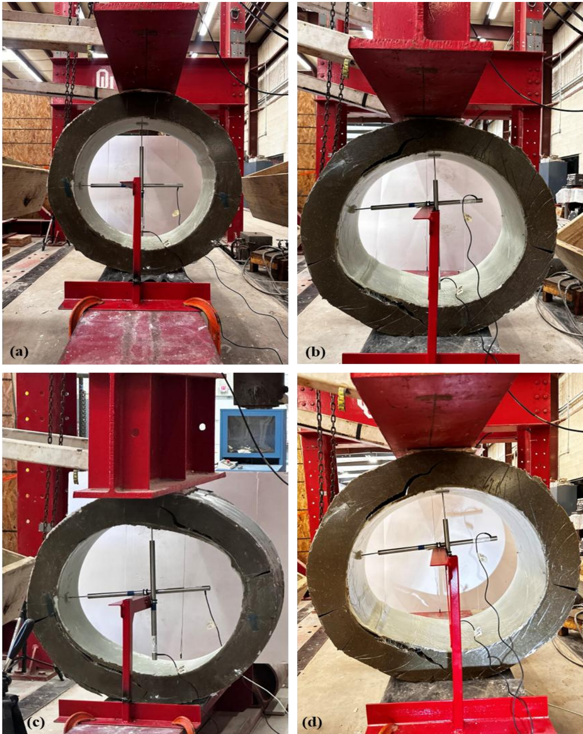
Figure 57: Uncorroded CMP with polymeric grout; (a) at the beginning of the test, (b) after failure; (c) and (d) symmetry of failure which happened in the pipes
