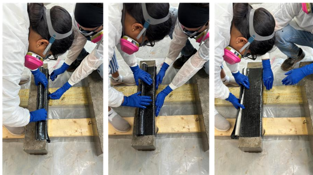
Figure 11: (a) Carbon fiber fabric wetting process for U-wrap. (b) Rolling wet fabric onto plastic pipe for layup on beam.
