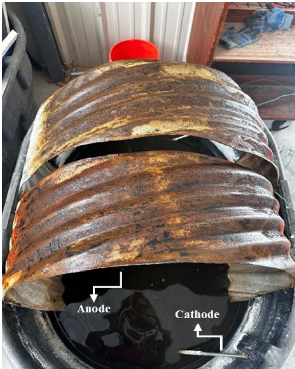
Figure 41: CMP specimens before and after three months of accelerated corrosion, showing the initial uncorroded sections in the tank, the corrosion setup with anode and cathode connections, and the resulting heavy rust concentrated at the crown region..
