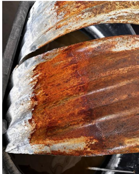
Figure 41: CMP specimens before and after three months of accelerated corrosion, showing the initial uncorroded sections in the tank, the corrosion setup with anode and cathode connections, and the resulting heavy rust concentrated at the crown region..
