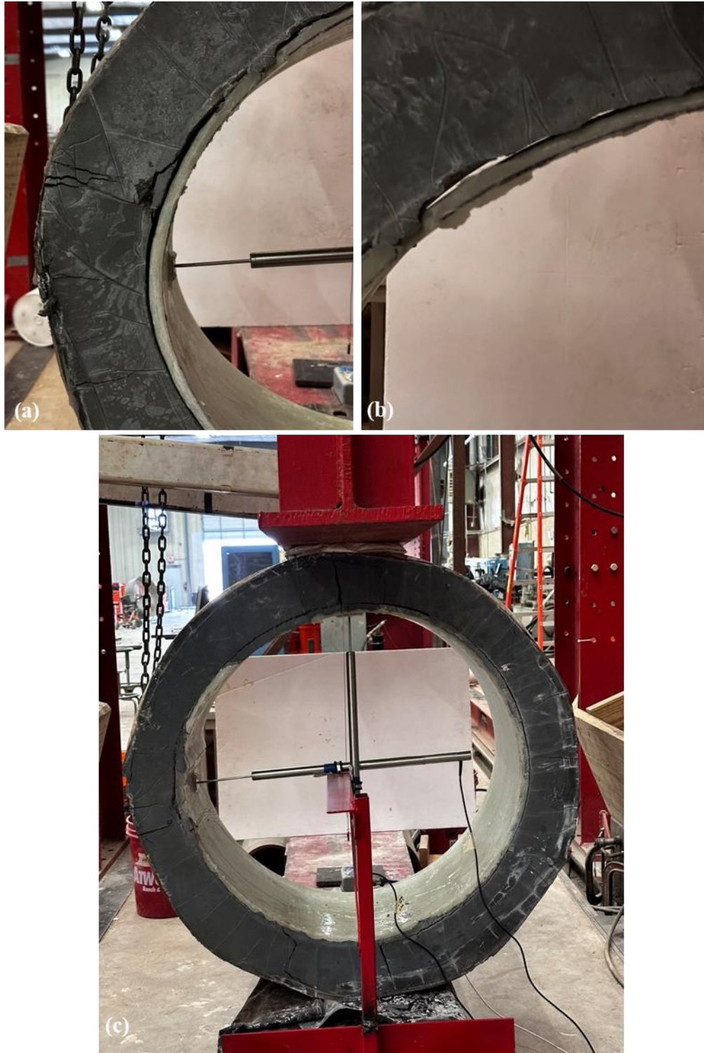
Figure 62: Pipes with cementitious grout after failure; (a) and (b) no bridging was observed between cementitious grout and GFRP pipe, (c) symmetry of failure
