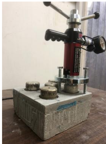
Figure 27: Preparation of the test specimens for the pull-off method (left–right), drilling cores, and the attachment of tensile loading devices.
