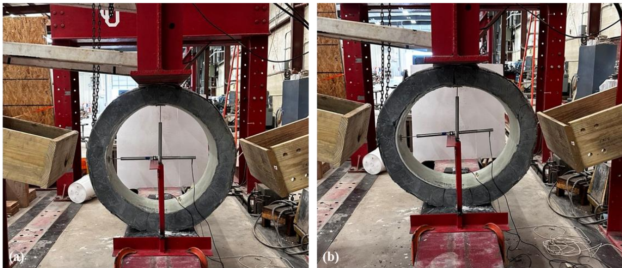
Figure 61: Uncorroded CMP with cementitious grout; (a) at the beginning of the test, (b) after failure
