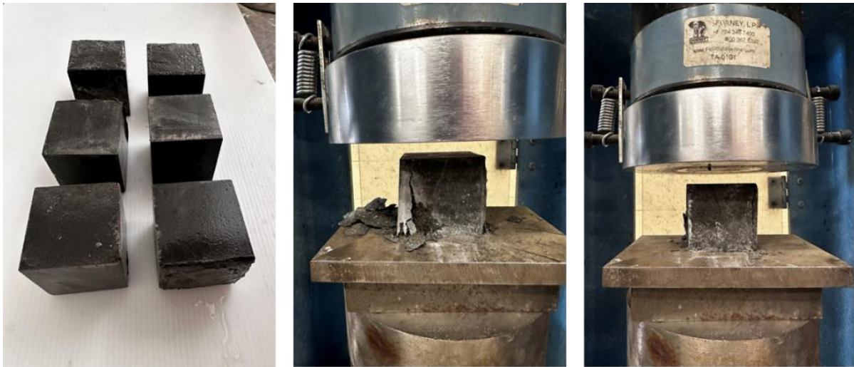
Figure 42: Cementitious grout specimens before and after failure.
