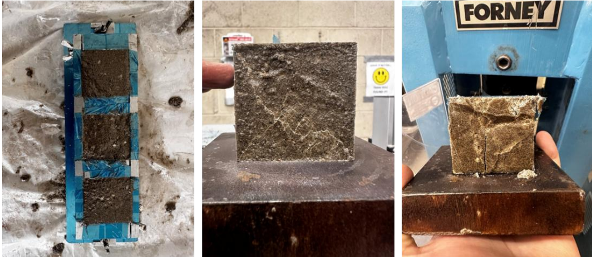
Figure 43: Polymeric grout specimens before and after failure.
