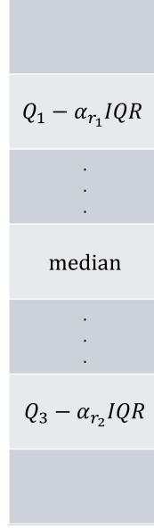
Figure 3.5: Visualization of the ordered data for an IQR-CFAR algorithm, with the threshold values highlighted. The training band is sorted into a column vector to determine the threshold.
