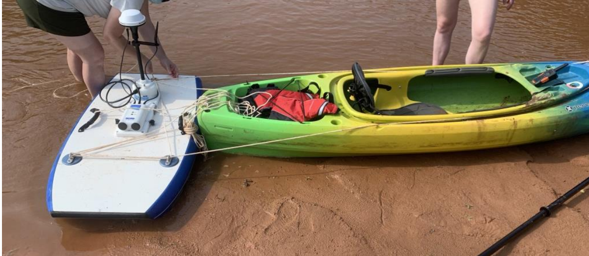
Figure 14: ADCP attached to back of kayak for cross sections in non-wadable rivers.
