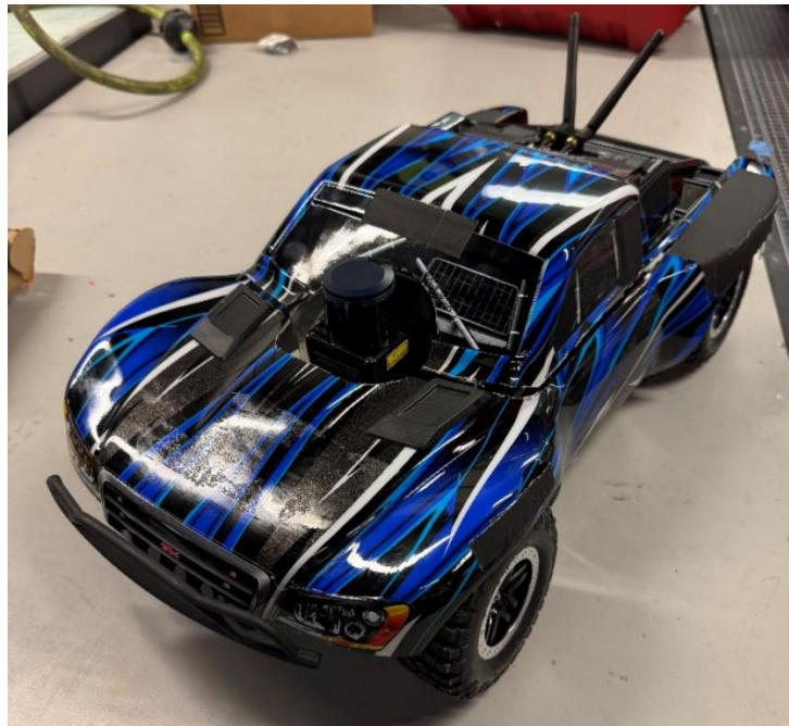
Figure 3-6: Completed SAGV Build with Cover
