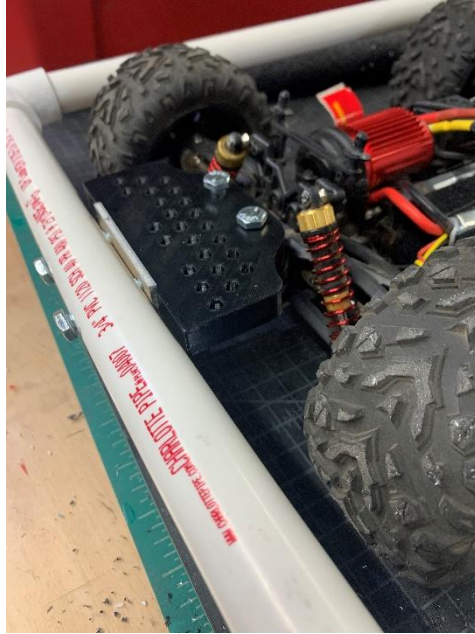
Figure 3.1-3: Top Side of Impact Area and PVC Pipes used as Bumper Frame
