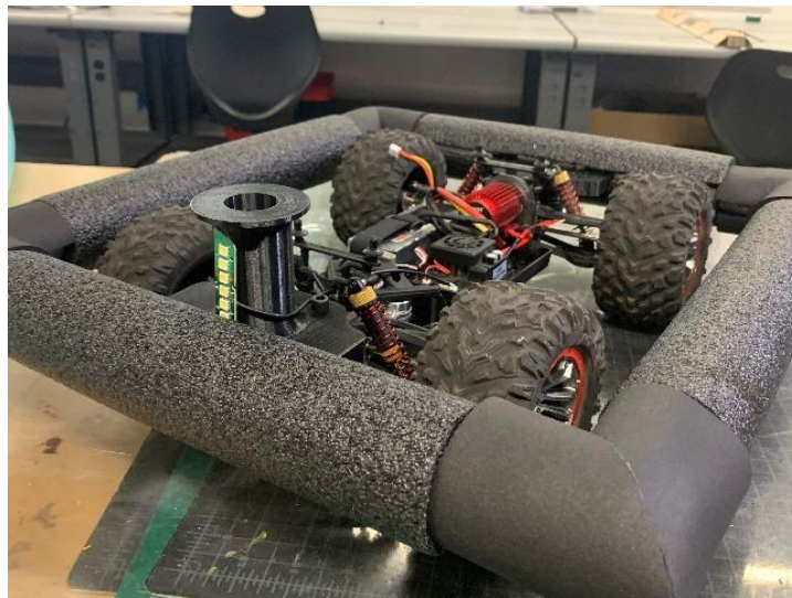
Figure 3.1-4: Assembled & Cushioned Bumper System and Pool Noodle Mount (part with lights)
