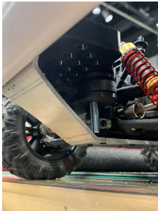
Figure 3.1-2: Impact Area (big black part) and Underside of Aluminum Mounting Bracket
