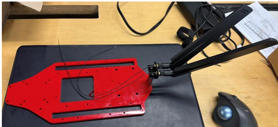
Figure 3.2.1-1: Platform Deck and Antennas
