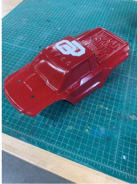
Figure 3.1-5: Trimmed and Painted Body for OU Softball (squares on sheet are 1/2" inch)
