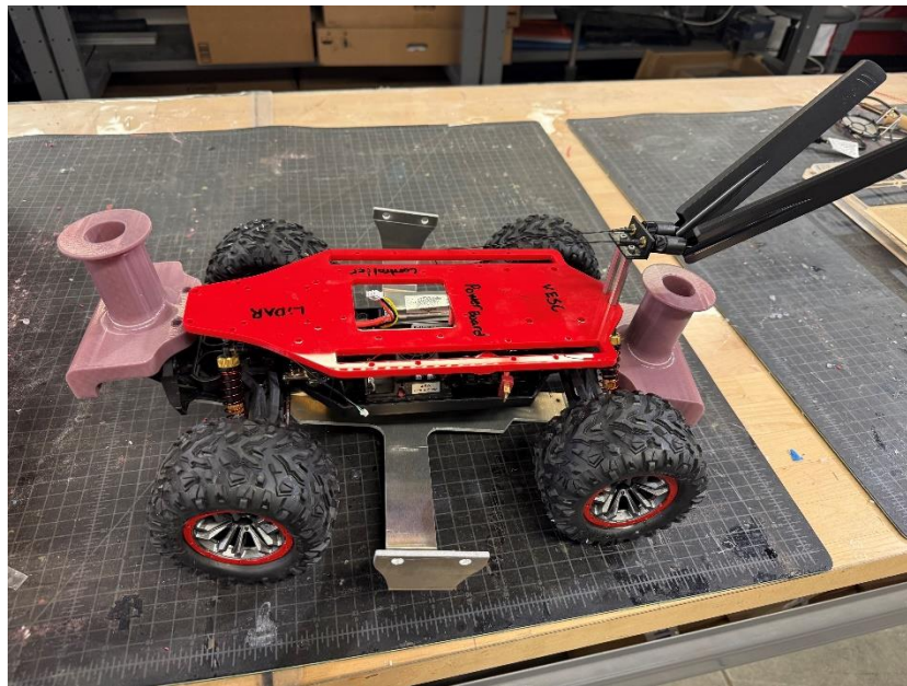
Figure 3.2.1-3: Mockup Assembly with Autonomy Stack and Bumper System on the HOSIM
