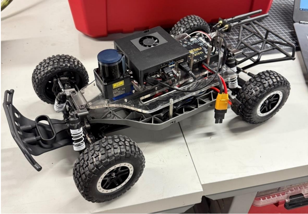
Completed SAGV Build No Cover
