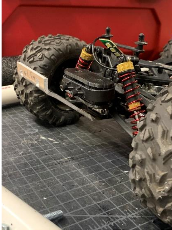
Figure 3.1-1: Front End of Aluminum Plate and Black Printed Parts for Impact Area
