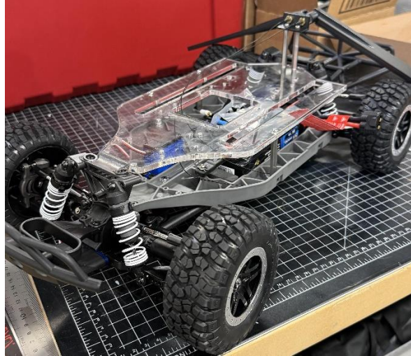
Figure 3-3: Torn Down Chassis with Platform Deck
