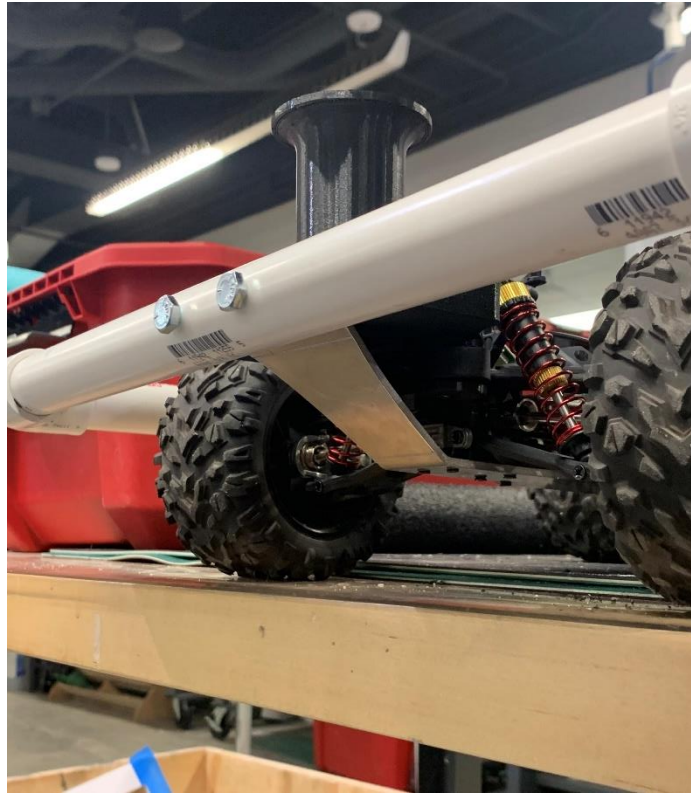
Undertray with Impact Area and Pool Noodle Mount
