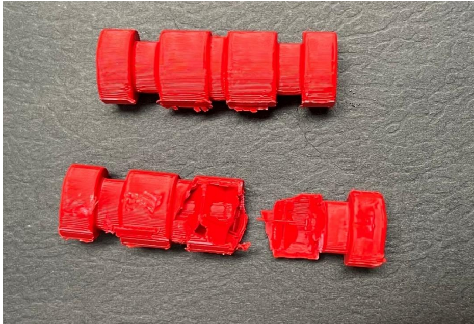
Figure 27: Intact Shear Pin and Fractured Shear Pin
