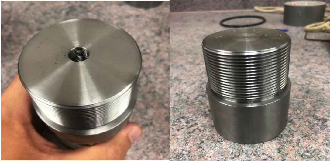
Figure 20. (a) Bottom view of flow cap with Swagelok threading (b) Replacement cap without openings.
