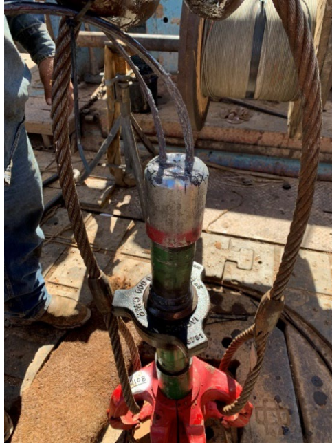
Figure 32. Tubing cap with the cable pass through.
