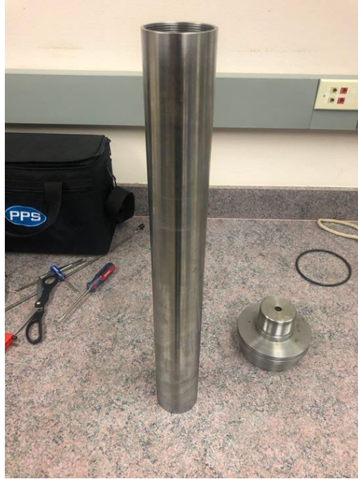
Figure 18. The fabricated tube of the housing.
