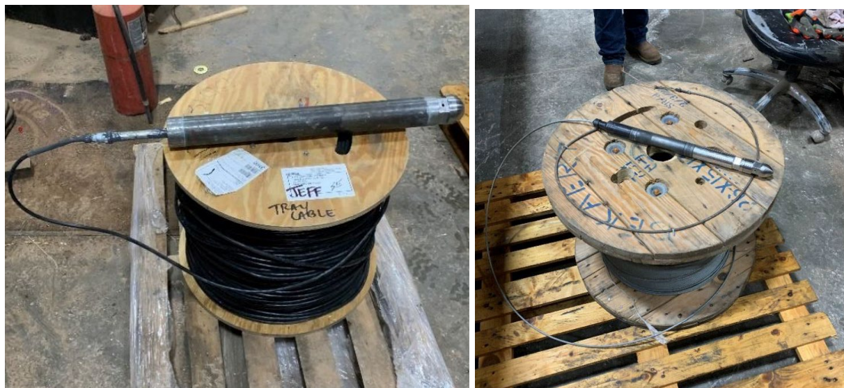
Figure 30. The all-digital sensor and reference sensor were connected to their cables.
