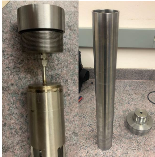
Figure 21. (a) Sensor assembled to the refurbished replacement cap. (b) Housing and the lid of the chamber.
