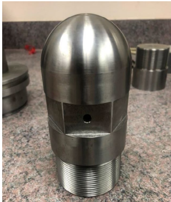
Figure 19. The fabricated flow cap of the housing.
