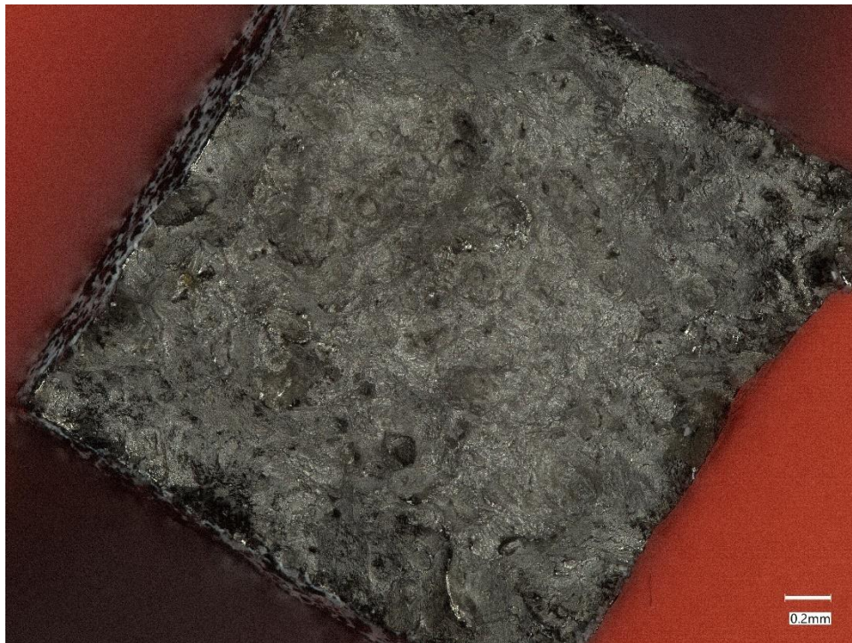
Figure 37: SR0 S1 Fracture Surface Top View 80x Depth Composition
