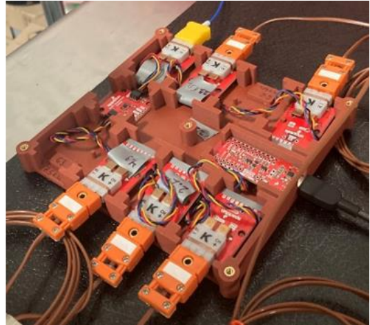
Figure 10: CAD of Thermocouple Housing and Completed Housing
