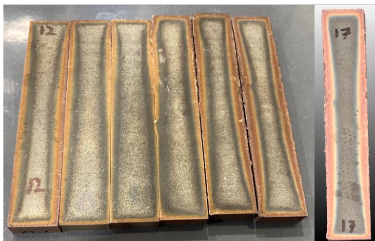
Figure 29: Bottom Face of SR1 After Heat Treatment
