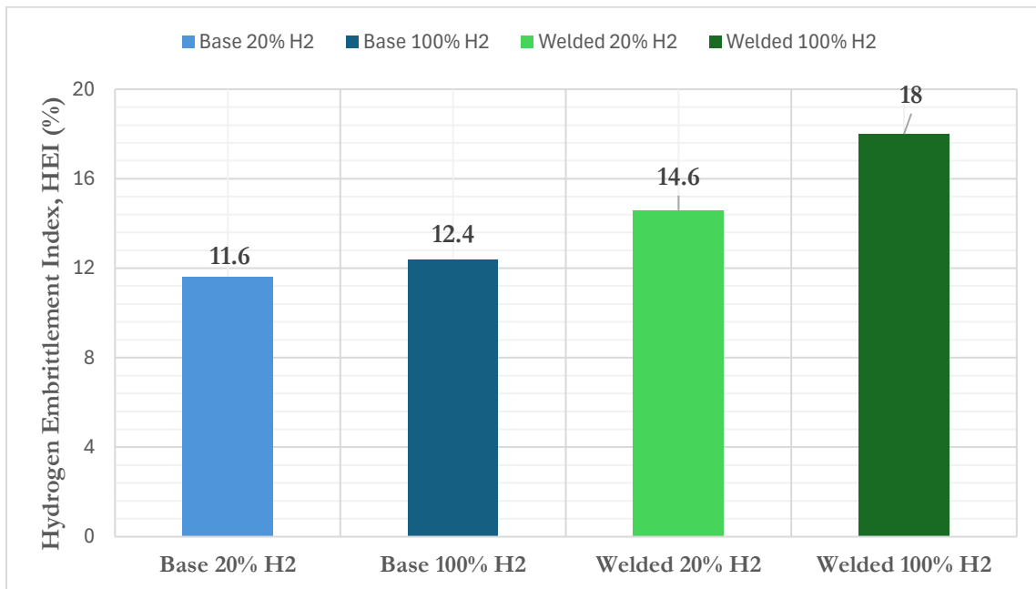
Figure 2-4 Hydrogen Embrittlement Index (HEI) of API 5L X60 base and welded materials at 20% and 100% H 2 at 2.07 MPa, measured by hollow-specimen slow strain rate tensile testing. Data sourced from [29].
