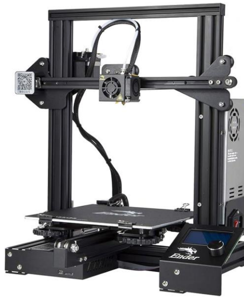
Figure 5. Unmodified Ender 3 FDM printer
