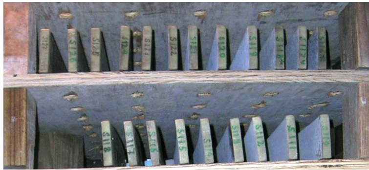
Figure 5.24 The specimens covered with curing compounds and stored in the chamber room
