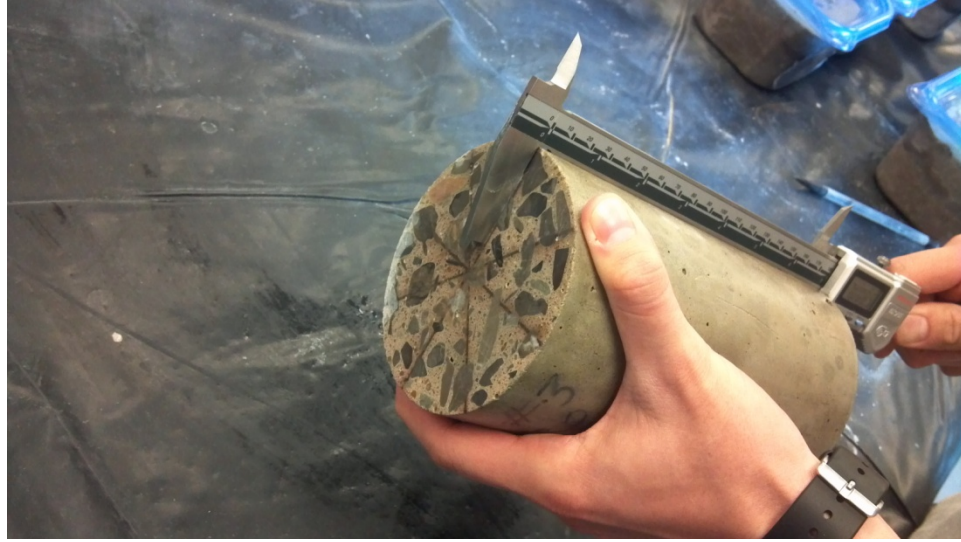
Figure 6.17 CTE cylinder during measurement with alignment markings
