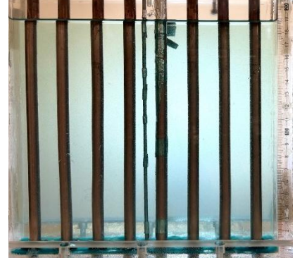
Figure 5-7 Temporal evolution of melting (discharging) for T_{\text{HTF, in}} = 55 \text{ }^{\circ}\text{C} and \dot{m}_{\text{HTF}} = 5 \text{ g/s} .
