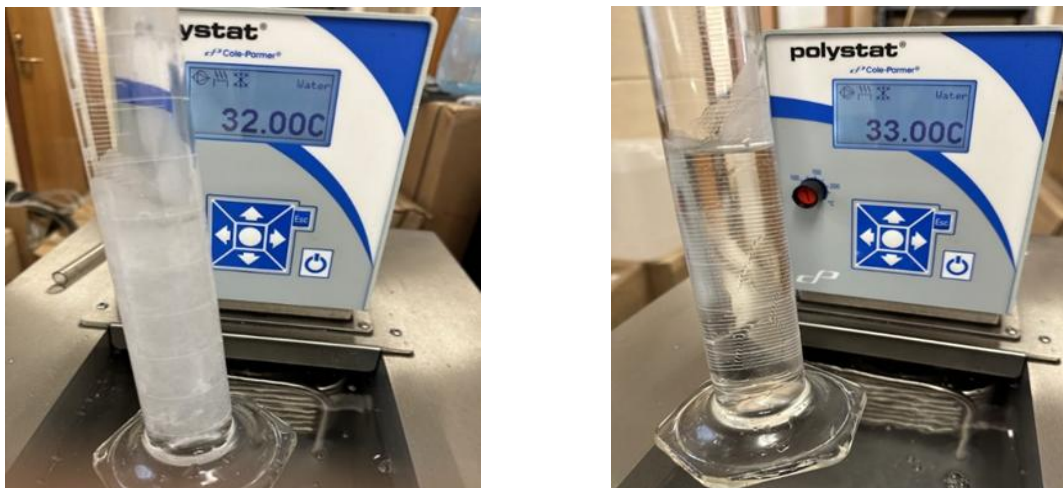
Figure 2-3 different stages of Melting of PCM using Polystat chiller and measured beaker.
