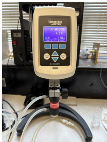
Figure 2-4 measuring the viscosity of PCM using Brookfield Ametek viscometer.
