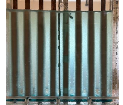
Figure 5-7 Temporal evolution of melting (discharging) for T_{\text{HTF, in}} = 55 \text{ }^{\circ}\text{C} and \dot{m}_{\text{HTF}} = 5 \text{ g/s} .
