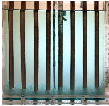
Figure 5-7 Temporal evolution of melting (discharging) for T_{\text{HTF, in}} = 55 \text{ }^{\circ}\text{C} and \dot{m}_{\text{HTF}} = 5 \text{ g/s} .
