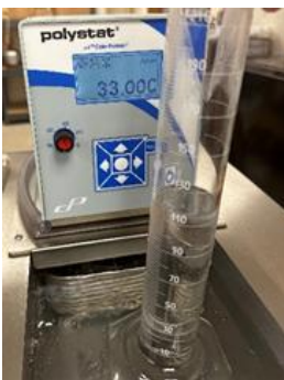
Figure 2-2 different stages of solidification of PCM using Polystat chiller and measured beaker.
