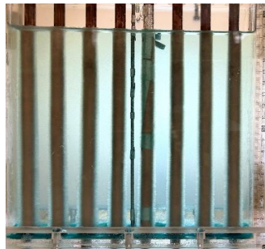
Figure 5-7 Temporal evolution of melting (discharging) for T_{\text{HTF, in}} = 55 \text{ }^{\circ}\text{C} and \dot{m}_{\text{HTF}} = 5 \text{ g/s} .
