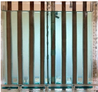
Figure 5-7 Temporal evolution of melting (discharging) for T_{\text{HTF, in}} = 55 \text{ }^{\circ}\text{C} and \dot{m}_{\text{HTF}} = 5 \text{ g/s} .
