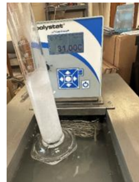
Figure 2-2 different stages of solidification of PCM using Polystat chiller and measured beaker.
