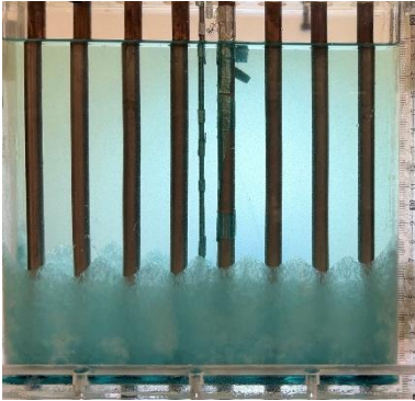
Figure 5-7 Temporal evolution of melting (discharging) for T_{\text{HTF, in}} = 55 \text{ }^{\circ}\text{C} and \dot{m}_{\text{HTF}} = 5 \text{ g/s} .
