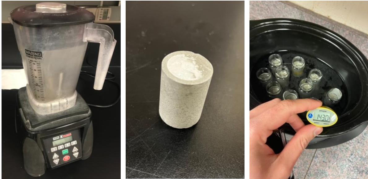
Figure 17. a) Blender used for mixing and cement sample preparation. b) Sample cylinder dimensions with a 1-inch diameter and 1.5-inch height. c) water bath for curing samples.
