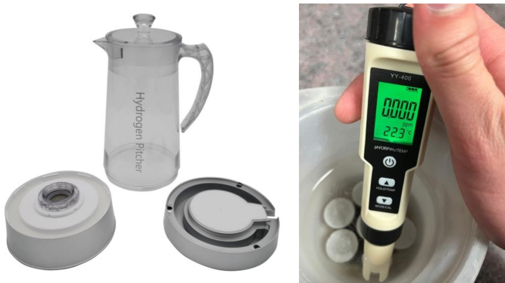
Figure 18. a) Hydrogen pitcher used to generate hydrogen in water. b) portable hydrometer used to measure hydrogen content in water in ppm, temperature in C, and pH.
