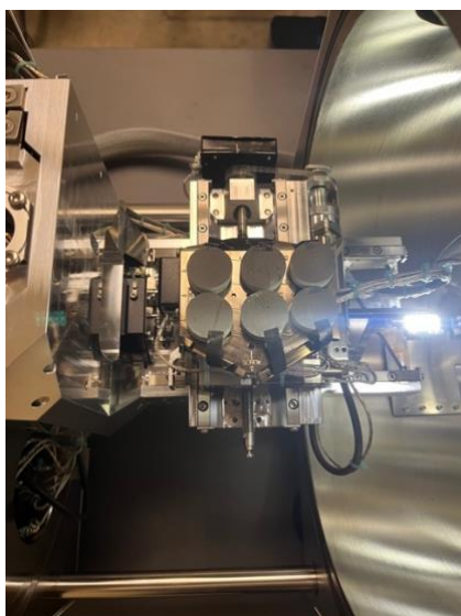
Figure 26. Thermo Quattro S field emission environmental Scanning Electron Microscope (FE-ESEM) used for Scanning Electron Microscopy (SEM) and Energy Dispersive X-Ray Spectroscopy (EDS). Cut samples placed before testing.
