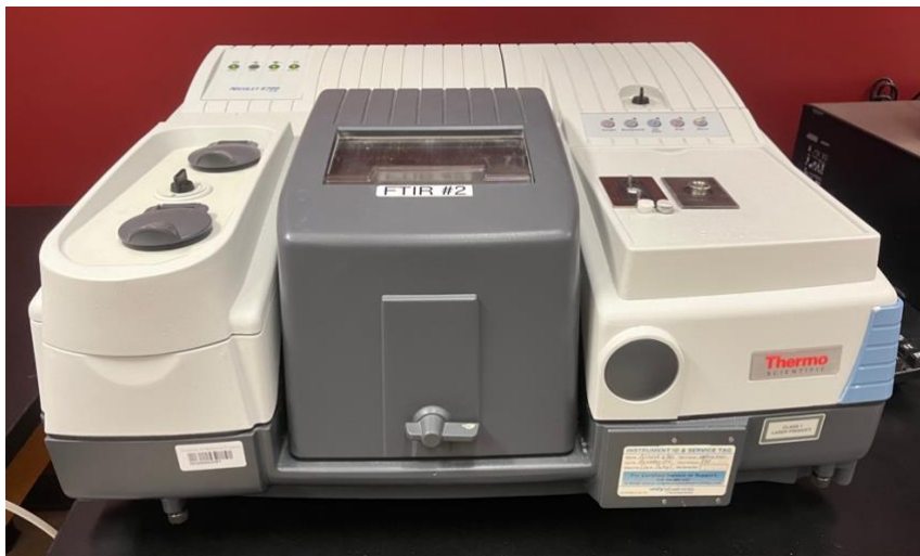
Figure 25. Nicolet 6700 Fourier Transformed Infrared Spectroscopy (FT-IR) Thermo Scientific equipment used to observe mineralogy.
