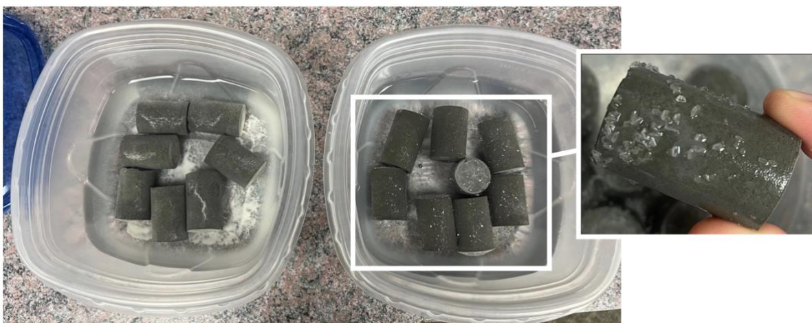
Figure 49. Samples after curing. The left is base water exposed samples, and the right is hydrogen exposed samples. It can be observed that hydrogen-exposed samples exhibit some crystals within the outer surface of the samples.
