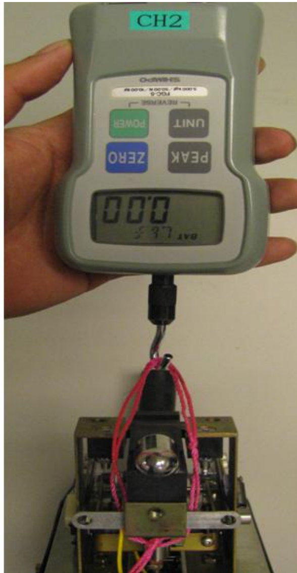
Figure 4.5: Setup for Calculating Stiffness of Plastic Hinges
