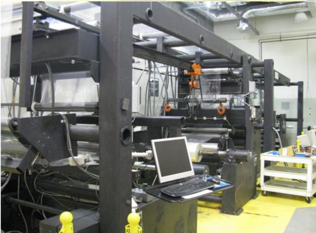
Figure 3.1: High Speed Winding Line – Web Handling Research Center, OSU
