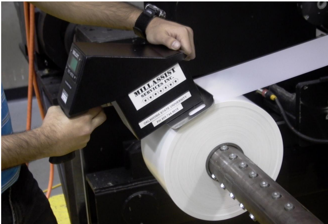
Figure 3.2: Hardness Measurement of Wound Roll using the Rho Meter
