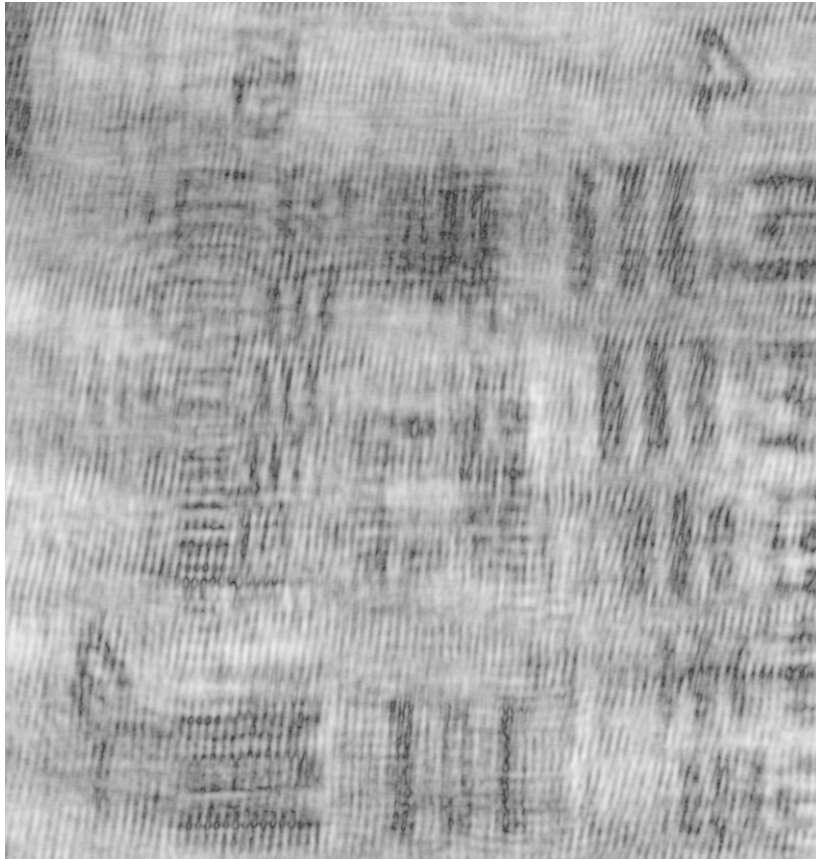
Figure 2-3 Reconstruction of a Resolution Target using the Digital In-Line Holographic Method with Magnification from a Relay Lens
