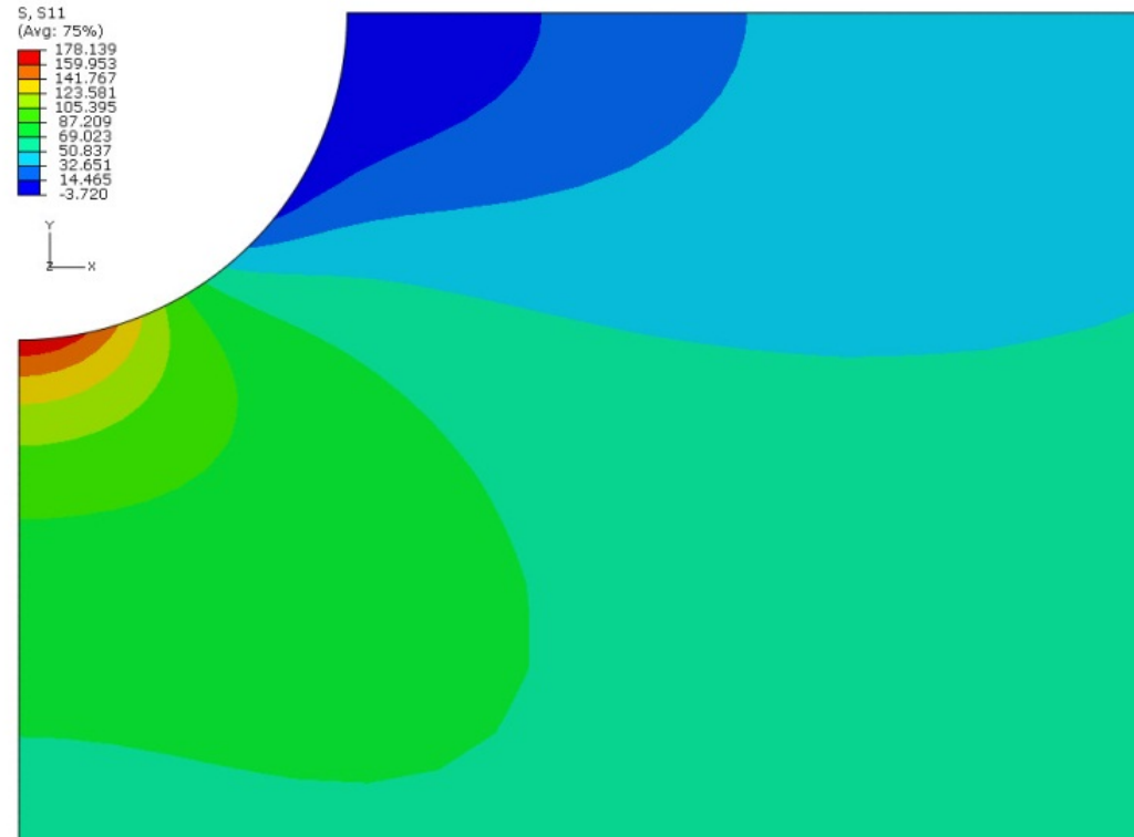
Figure 3 - Mesh size global .01 / local .005
