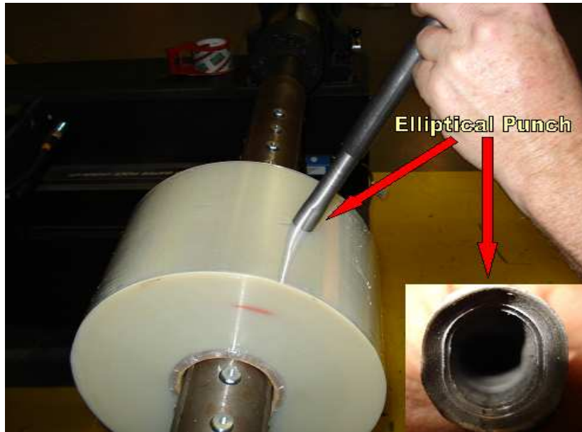
Figure 19 – Elliptical hole being punched in the roll.
