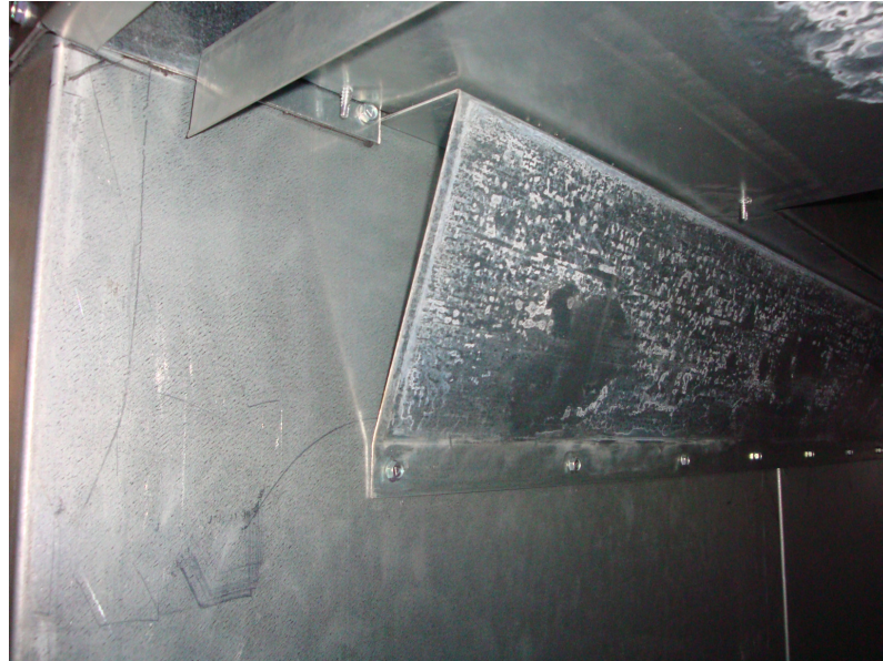
Figure 4.24: Triangular mounting bracket secured in code tester
