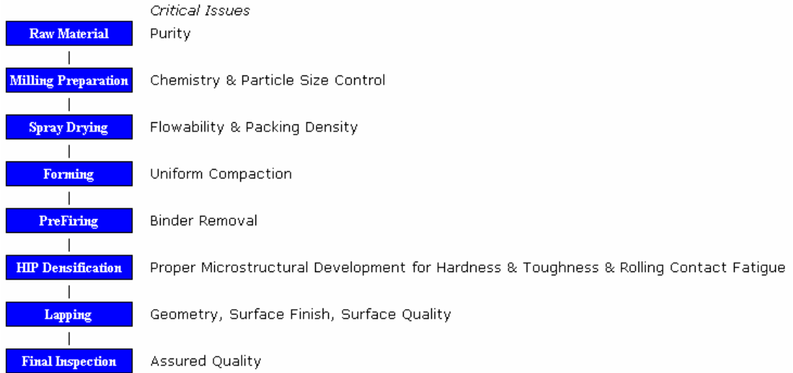
Figure 1.1.9 (In general) Commercial fabrication process for producing Si 3 N 4 balls [ http://www.cerbec.com/ ]
