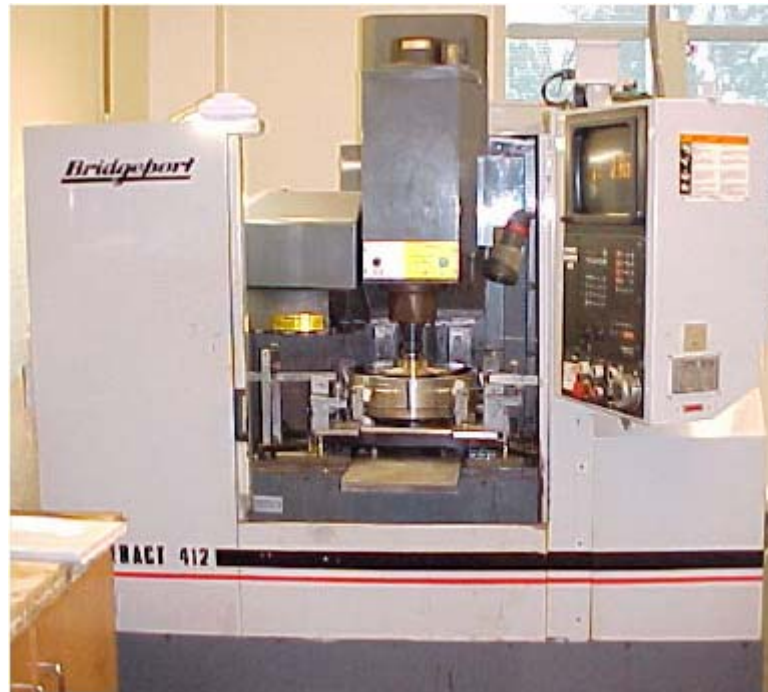
Figure 2.16 Photograph of a self-aligned large batch polishing apparatus used to finish larger \text{Si}_3\text{N}_4 balls (46 balls of 3/4 in. diameter) [Gerlick, 2004 and Kirtane, 2004]
