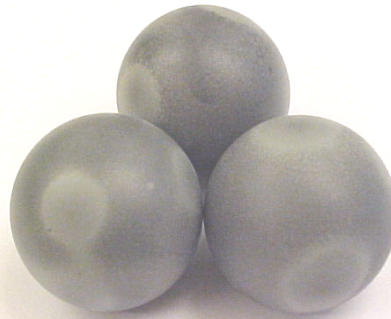
Figure 1.1.10 Photograph of the as-received (semi-finishing) Si 3 N 4 balls used in this investigation
