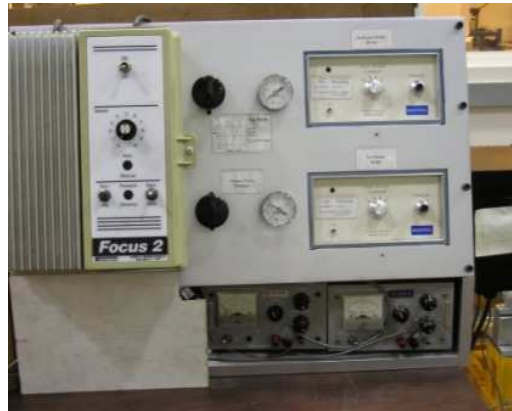
Figure 3.10: Master speed roller, nip roller, tacho-generator and its control panel
