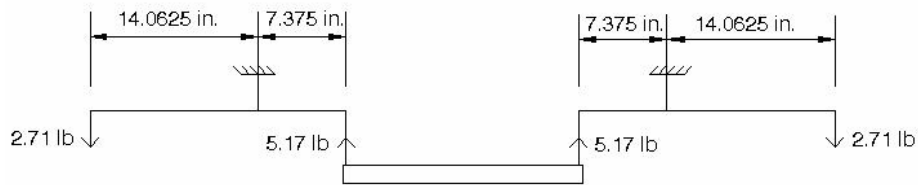
Fig. 4.17 Schematic showing the dimensions of the counterweight arm
