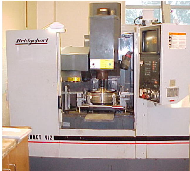
Fig. 4.2 Photograph of the machine tool used for polishing
