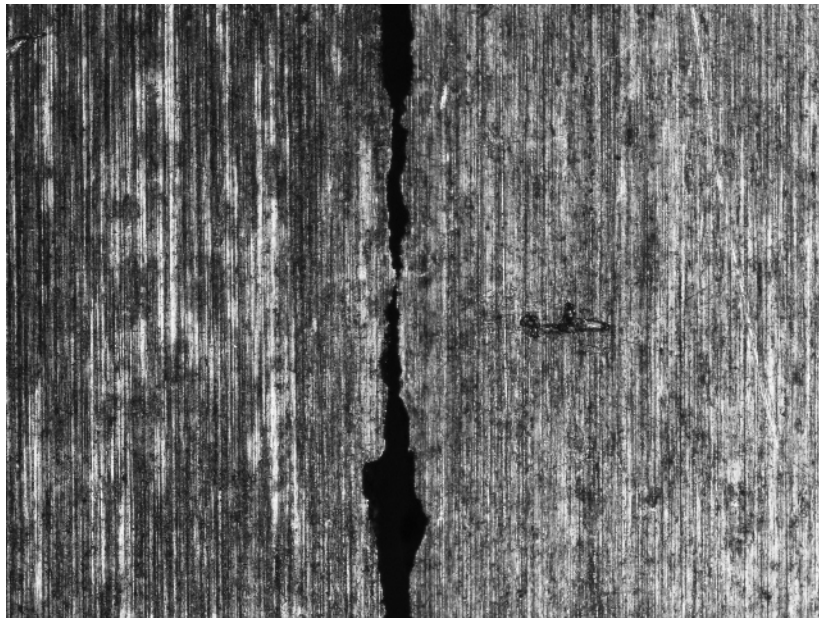
Figure 61 – 7075-T6 Corrode-During and Pre-Corroded (50x). The left specimen in the photo (T-70-4, N_f = 595,600 , Defl = 13 mm, 298 min) was corroded during cyclic loading and the right hand specimen (T-7P-4, N_f = 335,800 ) was pre-corroded 298 min. The specimen at left is notably more corroded than the one on the right; however the corrosion is general with no obvious pitting
