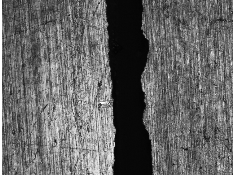
Figure 60 – 7075-T6 Corrode-During and Pre-Corroded (50x). The left specimen in the photo (T-70-1, N_f = 49,600 , Defl = 15 mm, 25 min) was corroded during cyclic loading and the right hand specimen (T-7P-1, N_f = 84,000 ) was pre-corroded 25 min. The difference between the two is negligible
