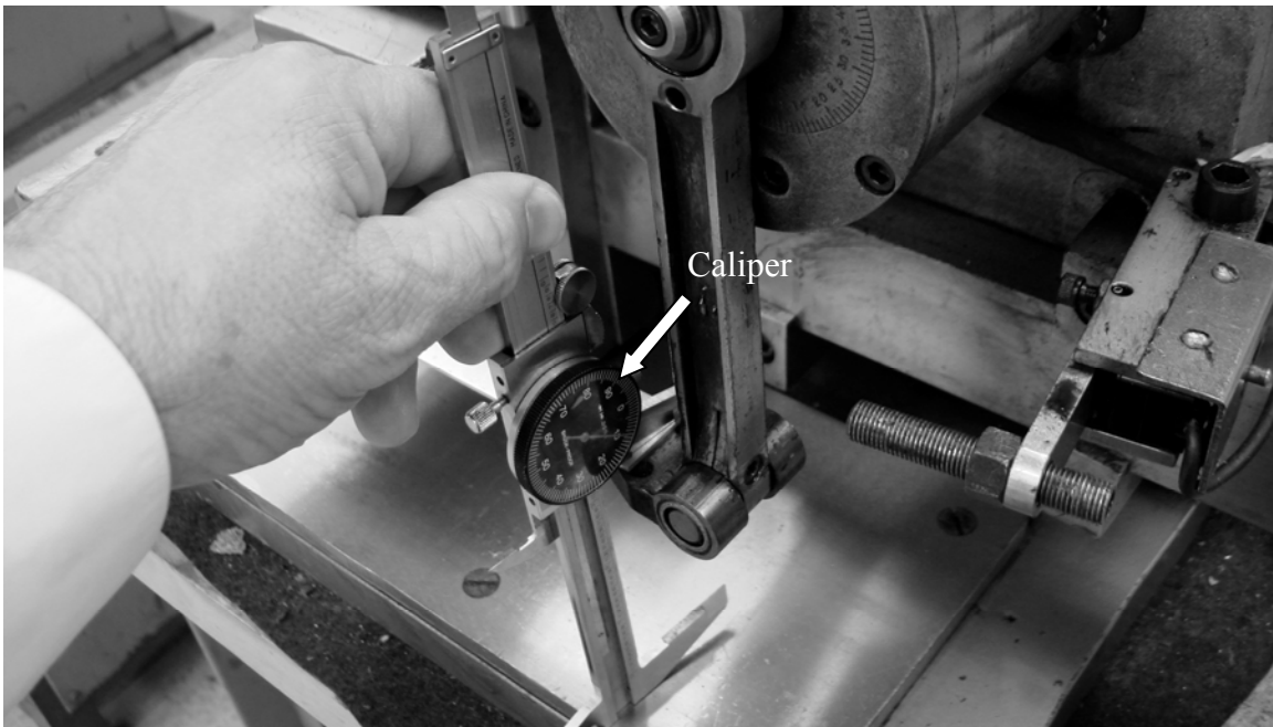
Figure 9 – Finding the upper most/null point of travel of the eccentric pivot rod. This measured value will be used to set the mounting block height to ensure the fixed end and mounted end of the specimen are level; a necessary condition for one-way bending.
