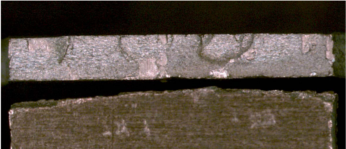
Figure 54 – Specimen T-9, 7075-T6 pre-corroded 30 minutes exposure to 15/1 ratio 3.5% NaCl solution to H 2 O 2 hydrogen peroxide, deflection = 15 mm (uncalibrated), N f = 51,300 cycles. (photo # TPS-002)
