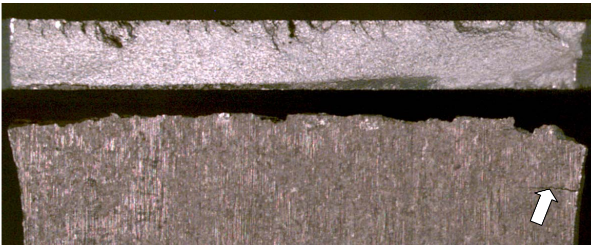
Figure 103 – Specimen LPH-4, 2024-T3 laser cut pre-corroded 10 minutes in a 30/1 ratio of 3.5% NaCl solution to H 2 O 2 hydrogen peroxide at 14 mm deflection, Nf = 73,200. Multiple ratchet marks (approximately 23 ea) can be seen originating at the top (tension) surface indicating multiple fatigue crack initiations – ratchet marks penetrate the surface about 1/3 -1/2 of thickness. One crack noted originating at the right-hand edge. (photo # LPHS-007)
