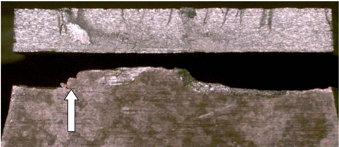
Figure 52 – Specimen T-7, 7075-T6, pre-corroded 60 minutes, exposed to 40/1 ratio 3.5% NaCl solution to H 2 O 2 hydrogen peroxide, deflection = 13 mm (uncalibrated), N f = 31,200 cycles. Cracks other than the primary fracture surface observable; one such is indicated by the arrow. Multiple ratchet marks indicate multiple cracks. (photo # TPS-005)
