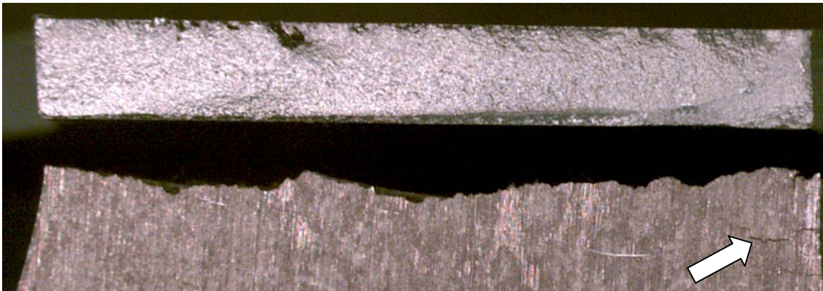
Figure 107 – Specimen LPH-5, 2024-T3 laser cut pre-corroded 5 minutes in a 30/1 ratio of 3.5% NaCl solution to H 2 O 2 hydrogen peroxide at 14 mm deflection, Nf = 114,900. Multiple ratchet marks (approximately 24 ea) can be seen originating at the top (tension) surface indicating multiple fatigue crack initiations – ratchet marks are relatively shallow and penetrate vertically into the surface less than about 1/4 of thickness on average. Two cracks noted by arrow, originating at the right-hand edge. (photo # LPHS-009)
