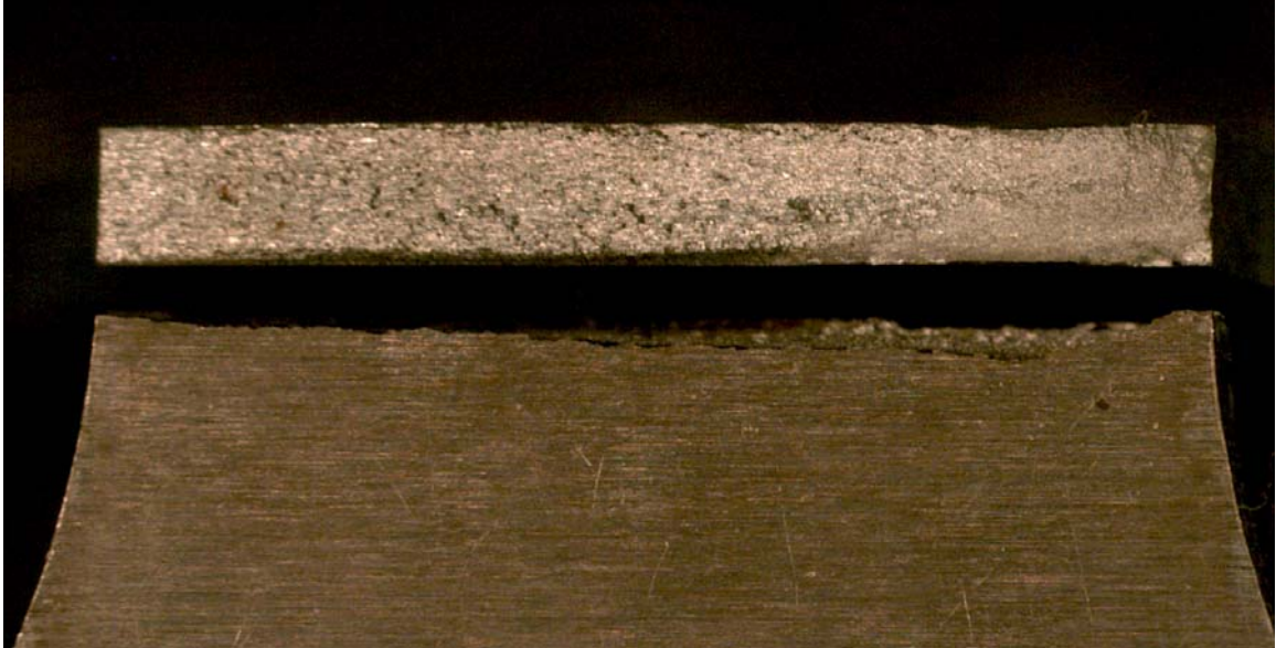
Figure 88 – Specimen 7PH-6, 7075-T6 pre-corroded 30 minutes in a 120/1 ratio of 3.5% NaCl solution to H 2 O 2 hydrogen peroxide at 14 mm deflection, Nf = 64,200. No discernable ratchet marks can be seen originating at the expected top (tension) surface – this is greatly reduced from the previous specimens indicating the minimum corrosion pitting value required to generate ratchet marks must be more severe. (photo # PHS-013)
