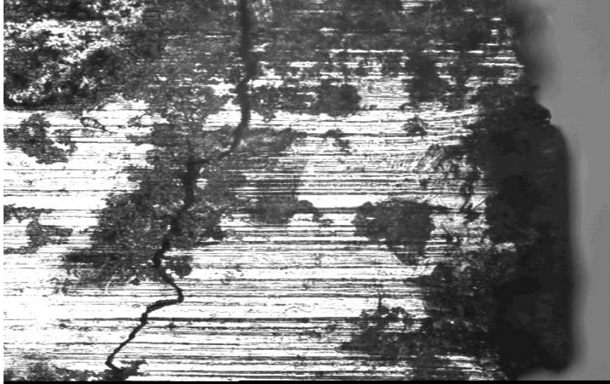
Figure 104 – Specimen LPH-4, 2024-T3 laser cut pre-corroded 10 minutes in a 30/1 ratio of 3.5% NaCl solution to H 2 O 2 hydrogen peroxide at 14 mm deflection, Nf = 82,000. Closer view (200x) of surface near fracture zone of Figure x above – a crack parallel to the fracture surface can easily be seen linking fields. (photo # LPH-009)
