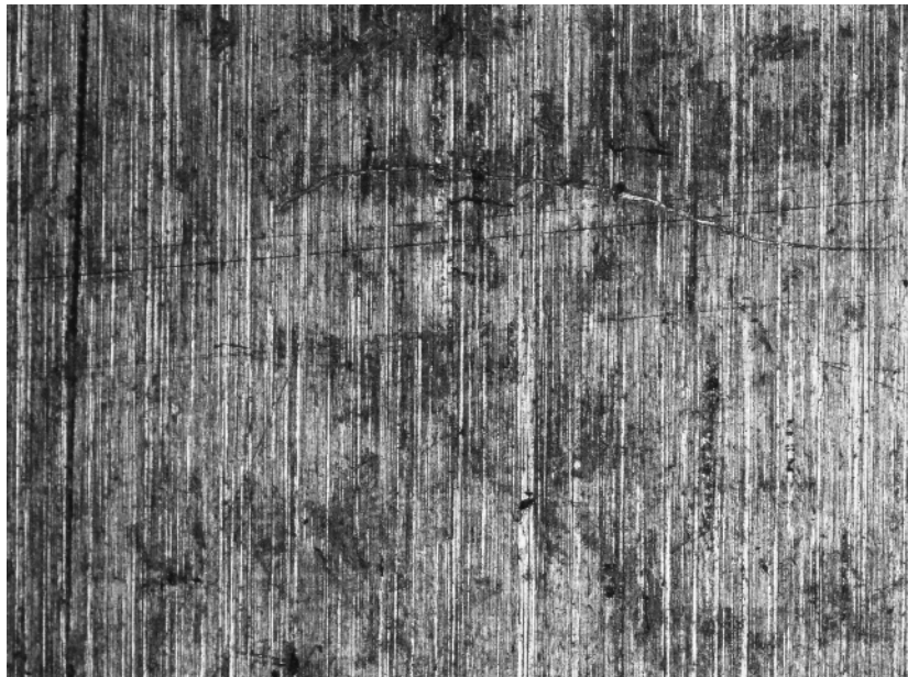
Figure 59 – 7075-T6, (50x) exposed to 400/1 ratio 3.5% NaCl solution to H 2 O 2 hydrogen peroxide, (uncalibrated). (a) Specimen T-14, N = 0 (uncycled), pre-corroded for 30.4 minutes. (b) Specimen T-13, cycled at deflection = 15 mm to Nf = 60,800 or 30.4 minutes. Severity of general corrosion slightly higher in (b) cycled vs. (a) uncycled. Initiation of a few pits is evident as well. Difference indicates cyclic loading may accelerate/worsen corrosion rate.
