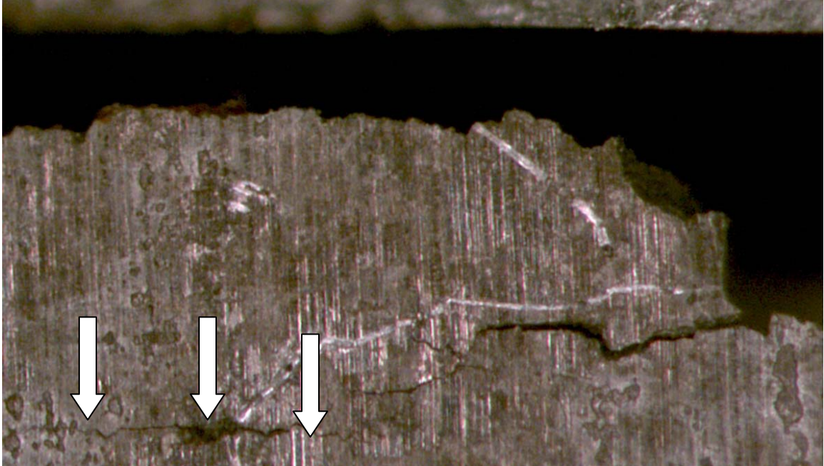
Figure 100 – Specimen LPH-2, 2024-T3 laser cut pre-corroded 70 minutes in a 30/1 ratio of 3.5% NaCl solution to H 2 O 2 hydrogen peroxide at 14 mm deflection, Nf = 73,200. Closer view (50x) of secondary cracks, noted in Figure x above, running parallel to primary fracture surface – arrows indicate another fatigue crack traversing left and right from a pit (center arrow); crack has not yet linked to the larger crack at right. (photo # LPHS-004)
