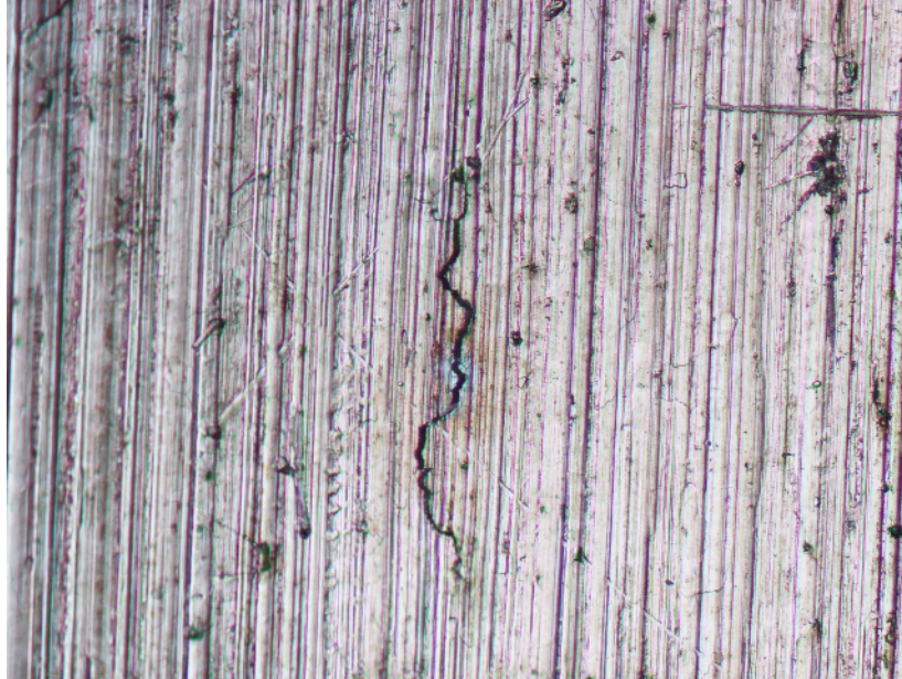
Figure 75 – T-60-3 Specimen (200x) 6061-T6, Defl = 17 mm, Nf = 42,500. Note the secondary crack off the primary fracture surface; source is not apparent but it could have occurred at an inclusion or constituent, exacerbated by corrosion-during cyclic loading. (photo NH-027)
