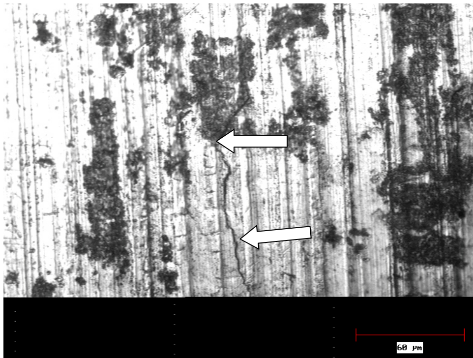
Figure 95 – Specimen 6PH-4, 6061-T6 pre-corroded 15 minutes in a 30/1 ratio of 3.5% NaCl solution to H 2 O 2 hydrogen peroxide at 14 mm deflection, Nf = 76,500. Crack can be seen running through corrosion pits away from primary fracture surface. (photo # PH-030)
