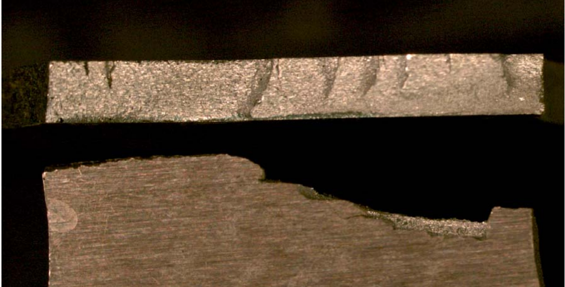
Figure 86 – Specimen 7PH-4, 7075-T6 pre-corroded 10 minutes in a 30/1 ratio of 3.5% NaCl solution to H 2 O 2 hydrogen peroxide at 14 mm deflection, Nf = 34,800. Multiple ratchet marks (approximately 9 ea) can be seen originating at the top (tension) surface. (photo # PHS-008)
