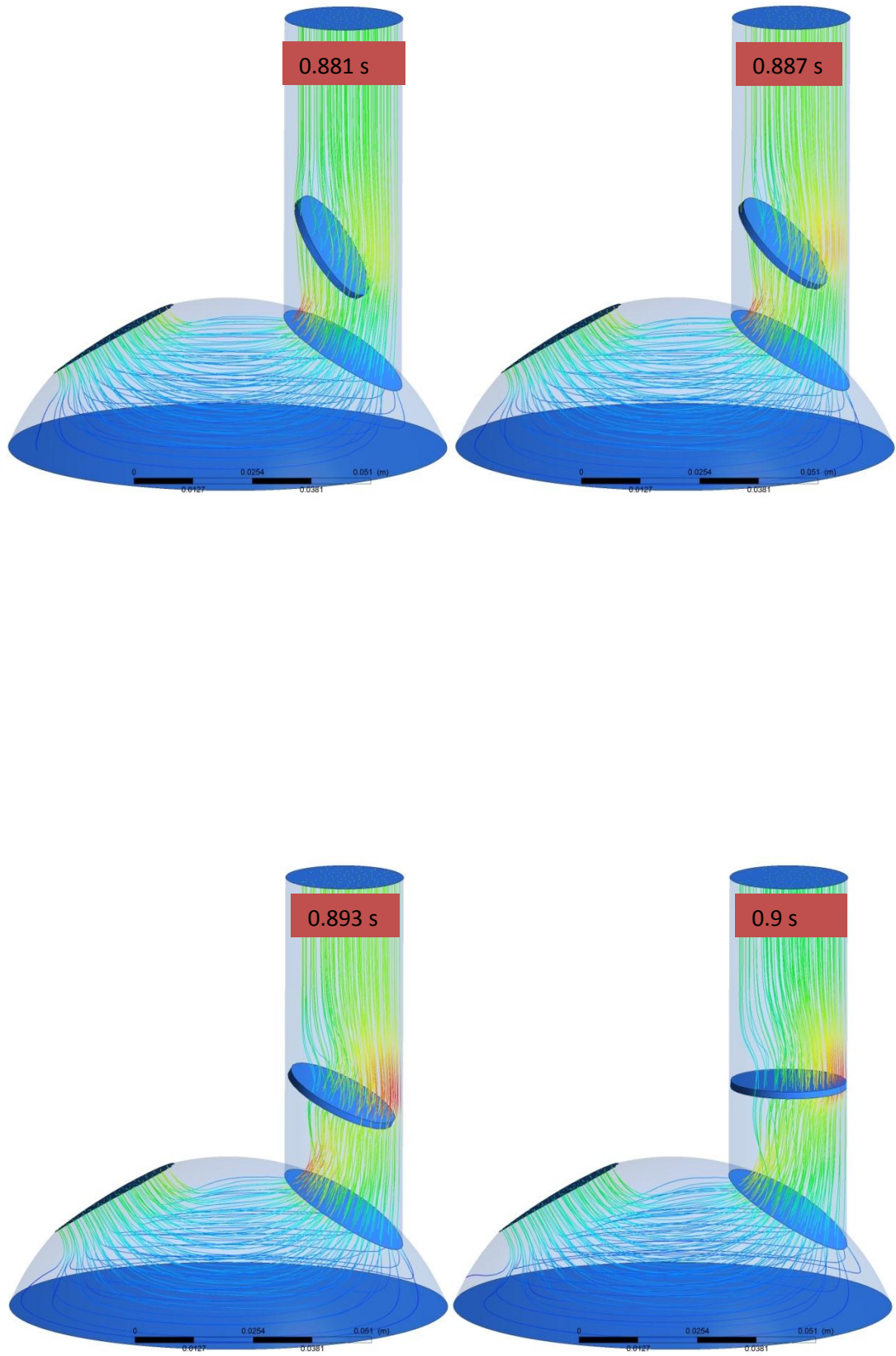
Figure 4.76 Velocity streamline during early systole when the monoleaflet inlet valve closes.
