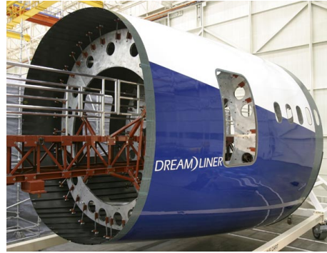
(b) Boeing 787 Dreamliner carbon fiber composite fuselage
