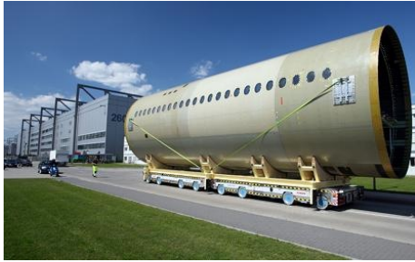
(a) Airbus A350 XWB carbon fiber composite fuselage
