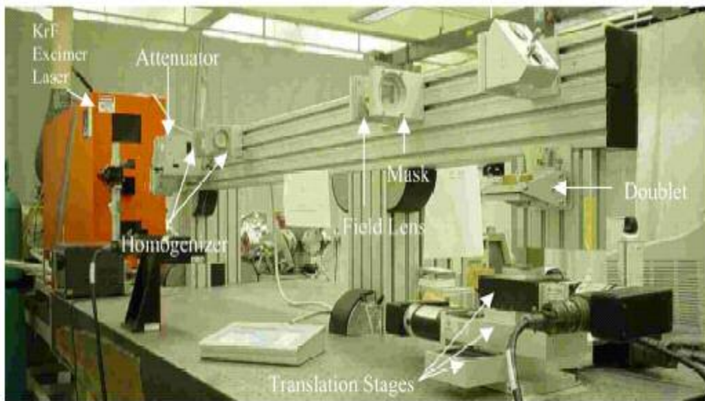
Fig.6.5 Photograph of the experimental setup used for laser micromachining [50].
