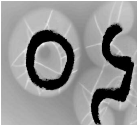
Fig 8.1 Transformation process from material build-up to material removal at 356 mJ energy
