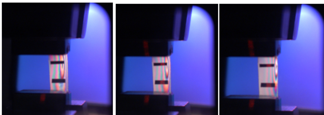
Figure 4.4: Fringes captured by low resolution Black & White Camera with its lens.
