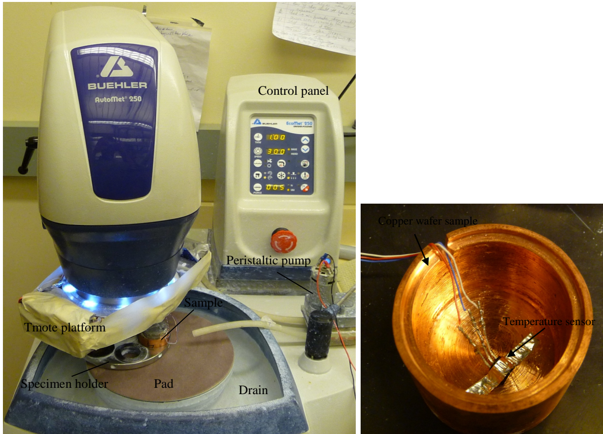
Fig. 4-6: (a) Buehler Automet 250 polishing machine (b) Copper wafer sample with a temperature sensor
