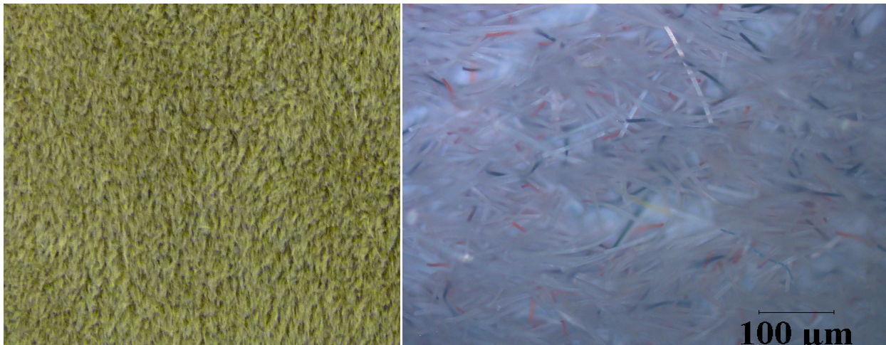
Intermediate pad, P_w = 0.6 , Fibers getting directional, nap decreased
