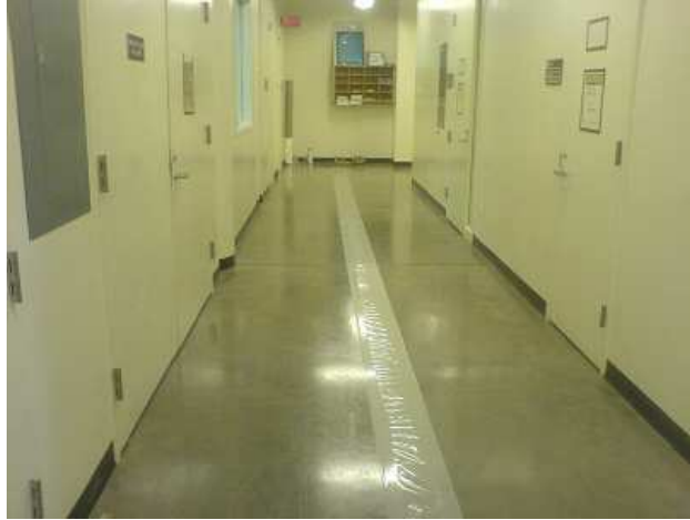
Figure 3.3- 60'' web stretched on the floor to run the stretch test
