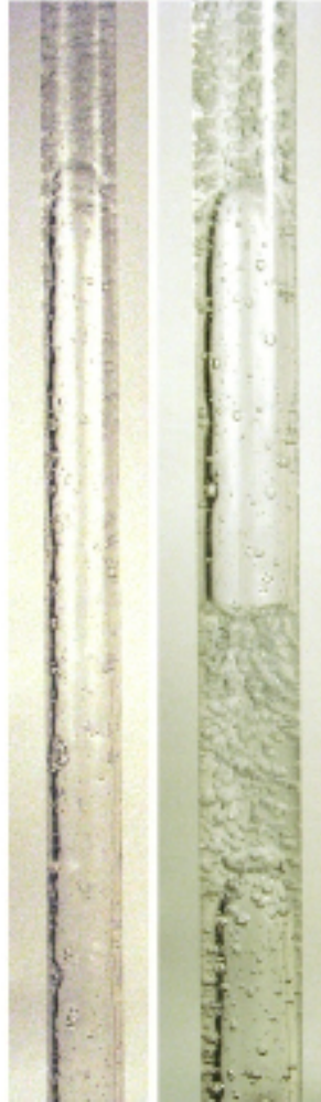
Figure 4.2 - Change in length of Taylor bubbles with increase in liquid flow
