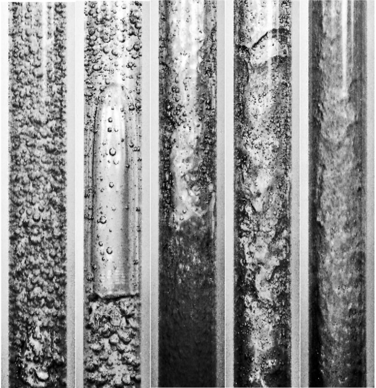
a) b) c) d) e) Figure 4.1 - Flow Patterns in Vertical Two-phase Flow a) Dispersed Bubble b) Slug c) Churn d) Froth e) Annular
