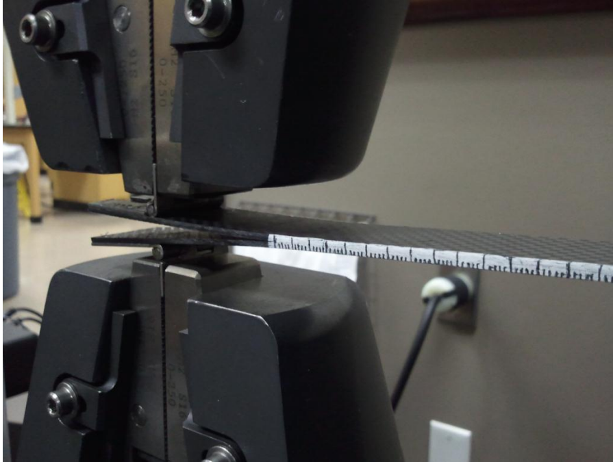
Figure 16: Double Cantilever Testing
