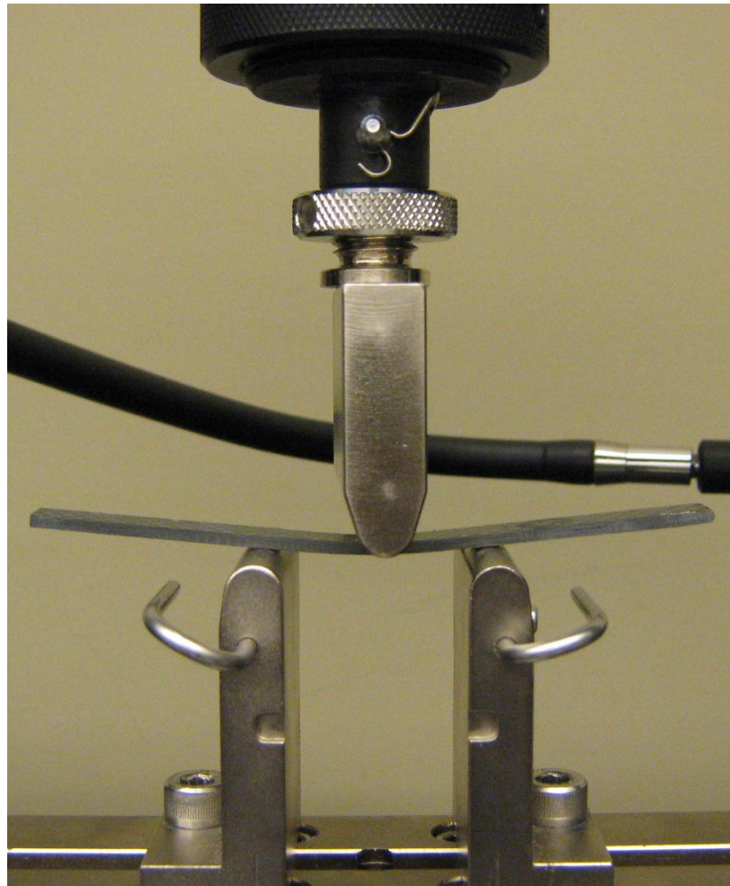
Figure 18: Flexure testing on the laminate
