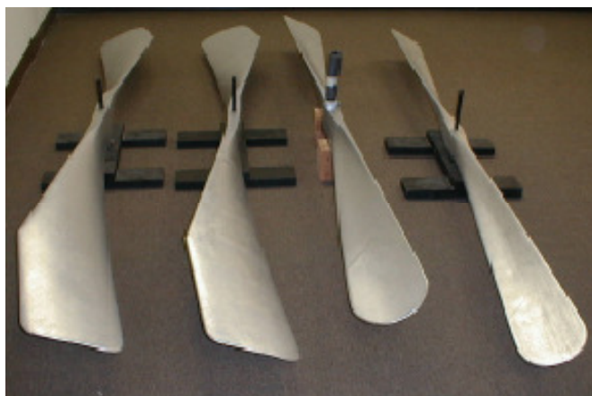
Figure 1: Photograph of Wright Brothers propeller reproductions between 1911 (left) and 1903 (right). Propeller lengths are 8 ft. 6 inches. 4
