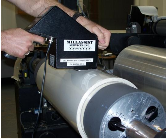
Figure 12 Taking hardness tests with Rho meter
