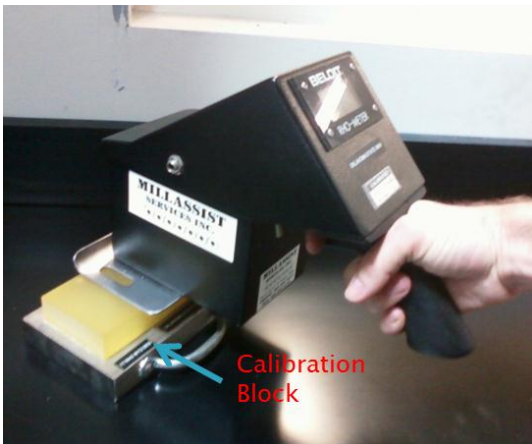
Figure 13 Rho meter on calibration block
