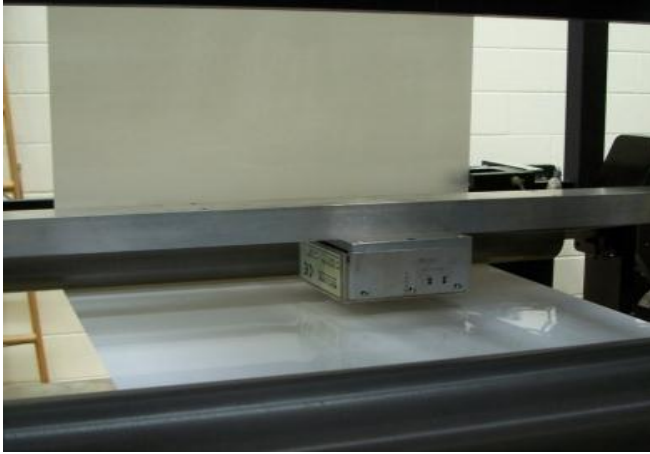
Figure 18 MeSys is mounted on a driven track
