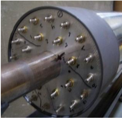
Figure 4 Variable resistors for balancing the sectors
