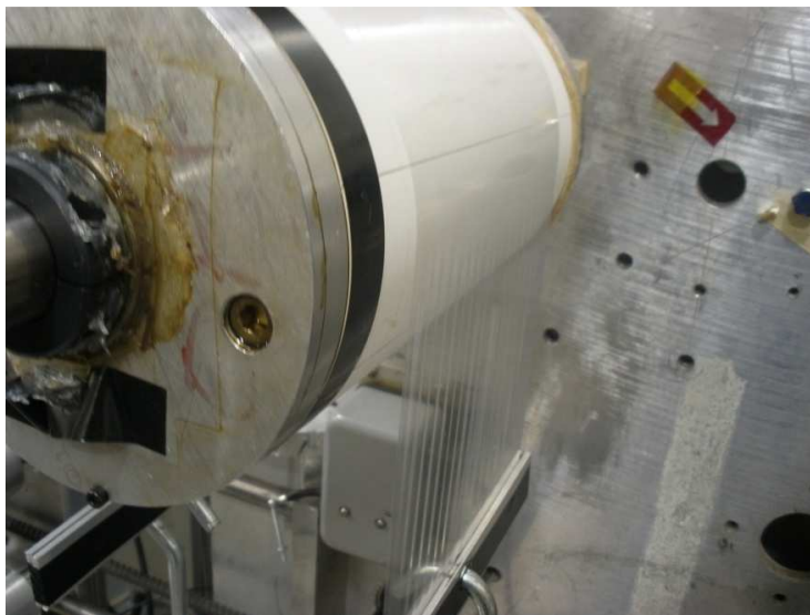
Fig 3.7: Troughs at the entry and exit, but no buckles on the roller (DOW 236) surface.
