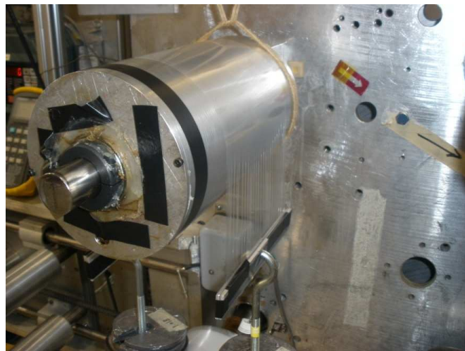
Fig 3.6: Troughs at the entry and exit, but no buckles on the roller surface.
