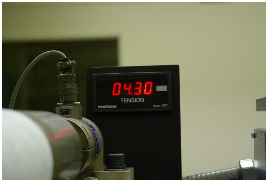
Figure 4.2: Tension Signal Conditioner and Display Unit in EWL
