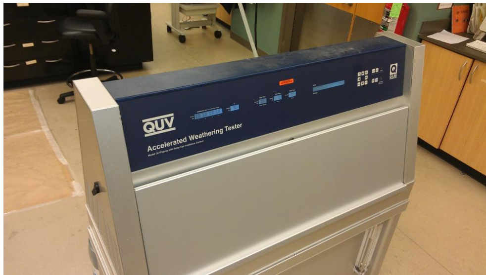
Figure 2.11: Test chamber used for alternating exposure of UV and condensation
