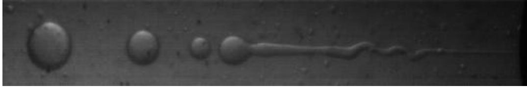
Figure 3.14 Flow irregularity resembling sinuous breakup mode of jet disintegration. We = 475 , We^* = 0.0115 .
