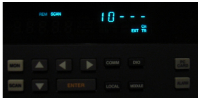
Figure D-4 Fluke –error status (need to reset Fluke before start operation)
