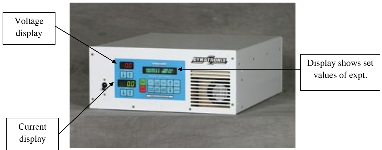
Fig. 2.1 Pulse Generator used for electrodeposition process
