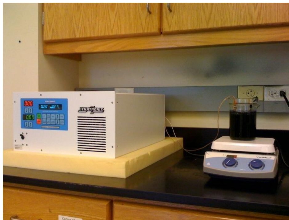
Fig. 2.3 Actual Experimental setup for electrodeposition process
