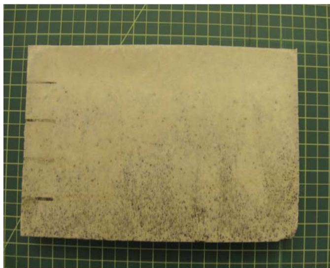
Figure 3.10: Rubber–polyurethane foam composites generated in this present study
