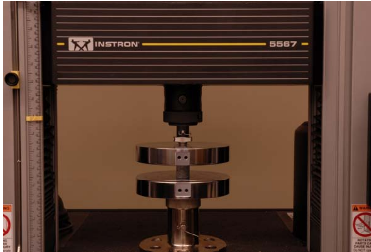
Figure 3.16: Foam–rubber specimens subjected to compression test following ASTM C365/C365M
