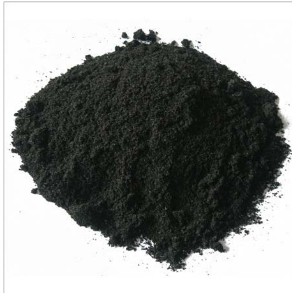
Figure 1.4: Typical crumb rubber particles recycled from waste tires, adapted from [15]
